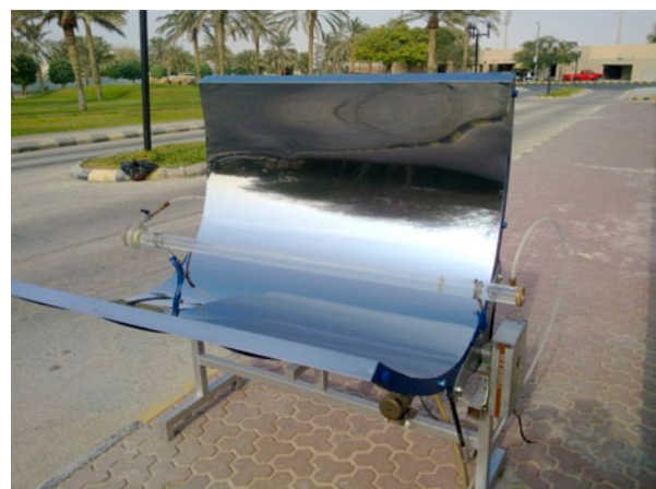
Fig. 4b. Pictorial view of experimental setup of PTC for photo catalysis.
