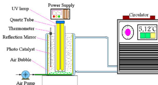
Fig. 1. A schematic diagram of the photoreactor setup.
