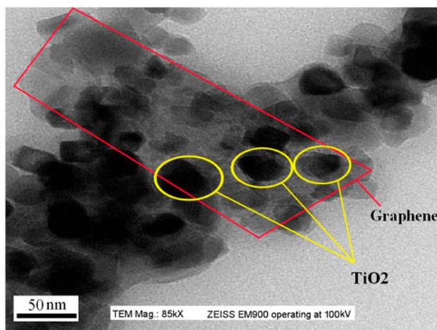
Fig. 2. TEM image of the TiO<sub>2</sub>/graphene hybrid.
