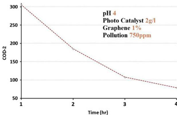
Fig. 3. COD decreasing over time under the optimum conditions.
