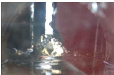
Fig. 17. Visualization of water surface flashing in the vessel. (The vessel temperature was 34.6 °C and the ambient temperature was 16.1 °C. The vacuum pressure was measured at 13.33 kPa (absolute).)
