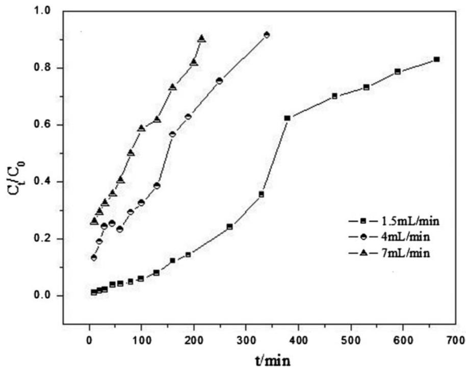
Fig. 3. The breakthrough curve of GRM column at different flow rates (MB initial concentration =  $150 \text{ mg L}^{-1}$ , column height = 14 cm).
