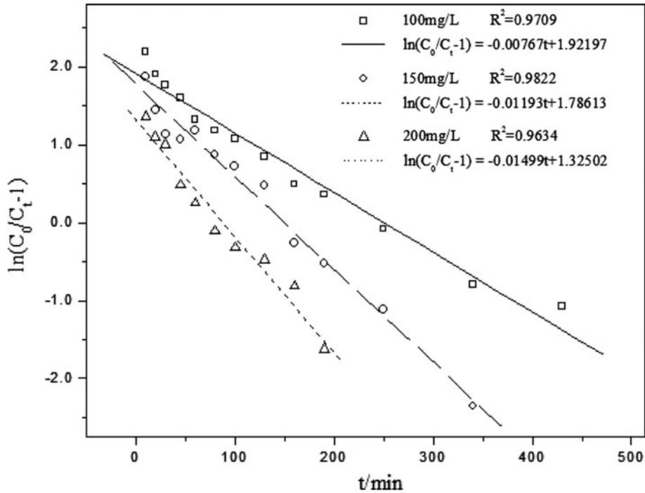
Fig. 7. The solution of Thomas model parameters for different MB initial concentrations.
