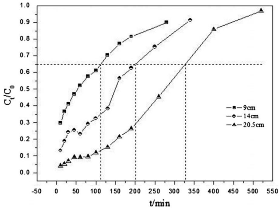
Fig. 2. The breakthrough curve of adsorption column for different packing column heights (MB initial concentration =  $150 \text{ mg L}^{-1}$ , flow rate =  $4 \text{ mL min}^{-1}$ ).
