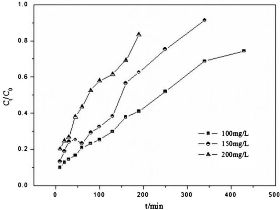
Fig. 4. The breakthrough curve of adsorption column under different initial concentrations (packing column adsorbent height = 14 cm, flow rate = 4 mL min<sup>-1</sup>).
