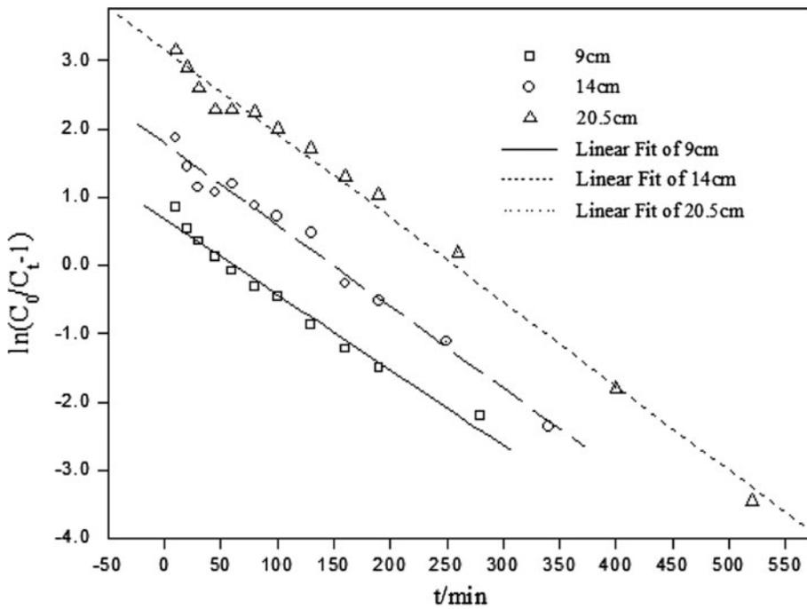
Fig. 5. The solution of Thomas model parameters for different bed heights.
