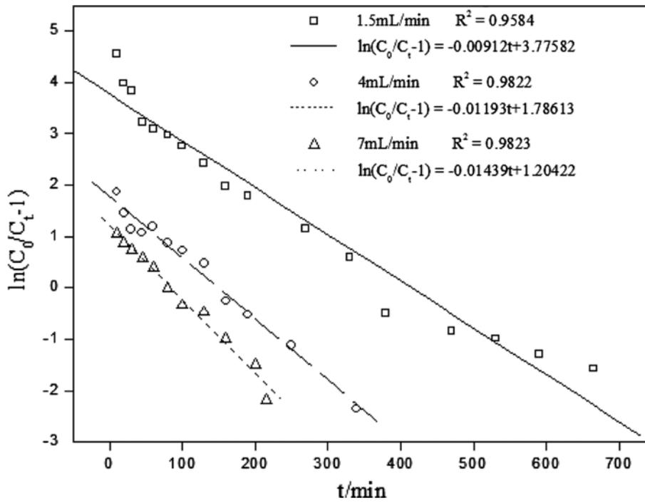
Fig. 6. The solution of Thomas model parameters for different flow rates.
