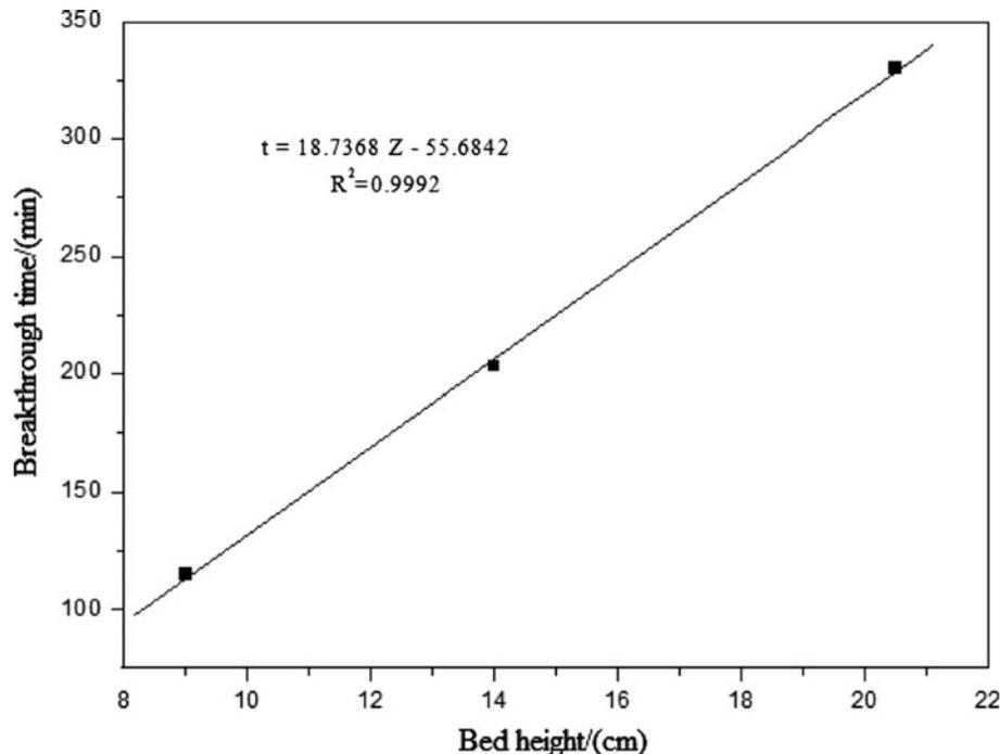
Fig. 8. The solution of BDST model parameters.
