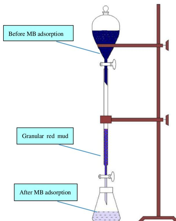
Fig. 1. Device connection diagram.
