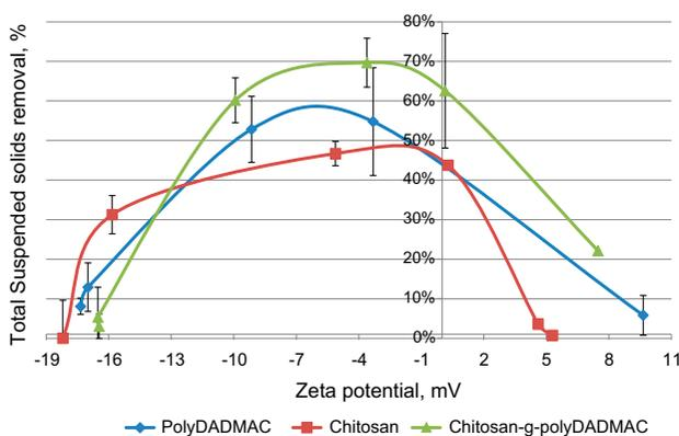
Fig. 5. Correlation between zeta potential and % TSS removal from Logan lagoon wastewater using polyDADMAC, chitosan, and chitosan-g-polyDADMAC.
