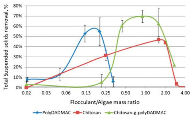
Fig. 4. Comparison of % TSS removal from Logan lagoon wastewater using polyDADMAC, chitosan, and chitosan-g-polyDADMAC.
