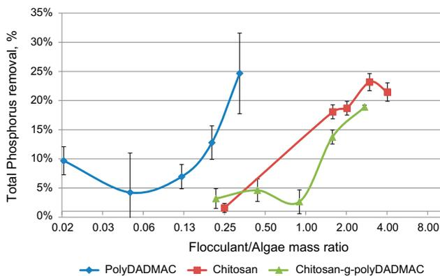
Fig. 7. Comparison of TP removal from Logan lagoon wastewater using polyDADMAC, chitosan, and chitosan-g-polyDADMAC.
