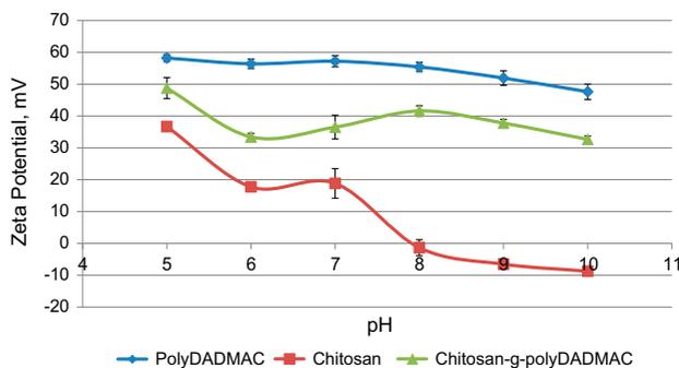
Fig. 2. Zeta potential titration curve for polyDADMAC, chitosan, and chitosan-g-polyDADMAC.
