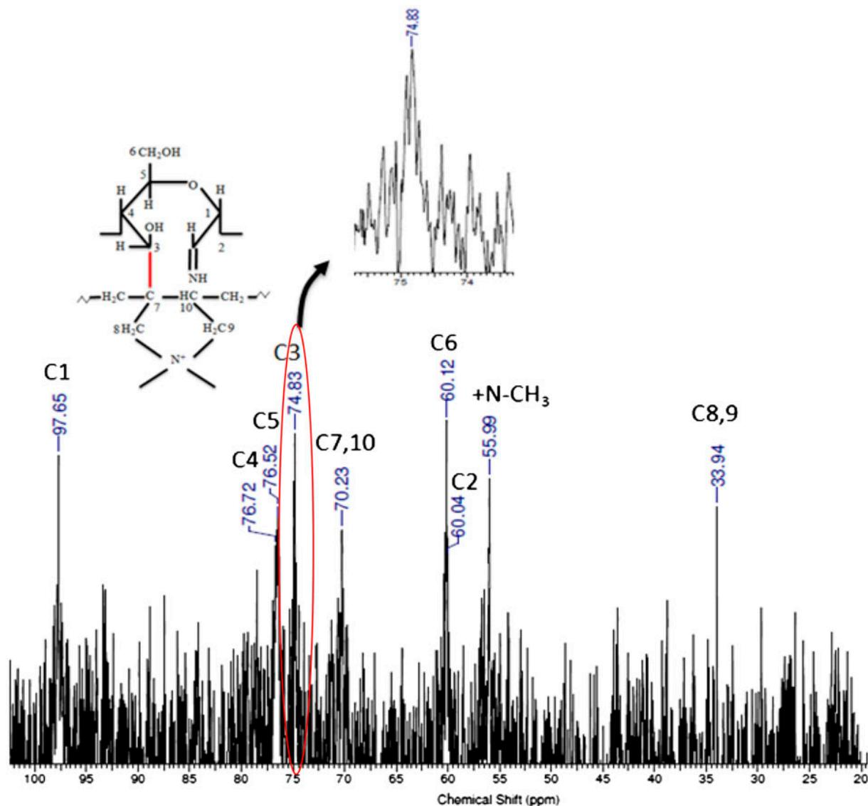
Fig. 3.  $^{13}\text{C}$ -NMR spectra of chitosan-g-polyDADMAC measured in  $\text{D}_2\text{O}$  (1% HCl) at 298 K.
