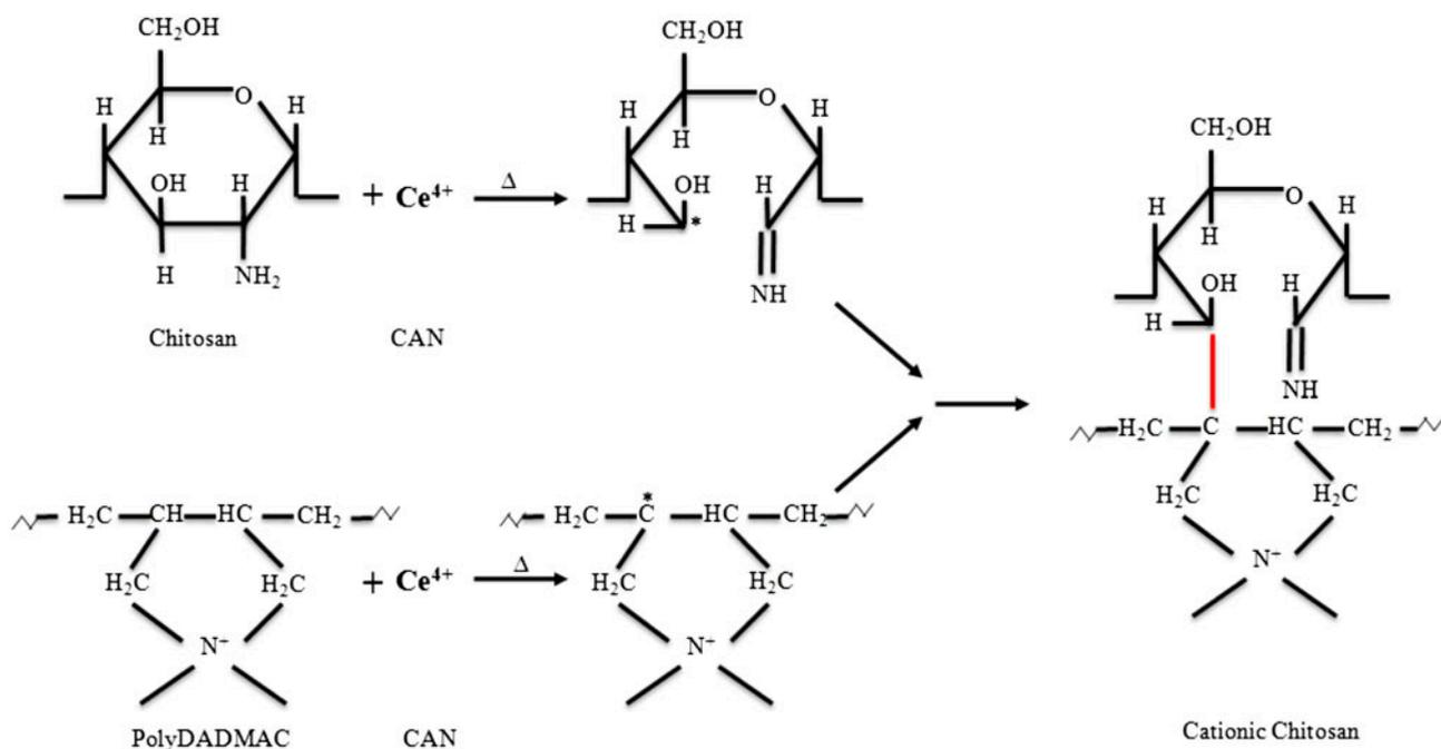
Fig. 1. General reaction scheme of grafting polyDADMAC onto chitosan.
