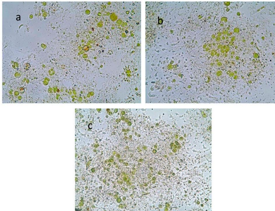
Fig. 6. Microscopic images (40 $\times$ ) of aggregates formed during the jar test for (a) polyDADMAC, (b) chitosan, and (c) chitosan-g-polyDADMAC.
