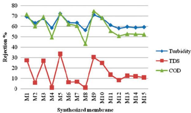
Fig. 7. Rejection percentages of the pollution indices vs. prepared membranes.
