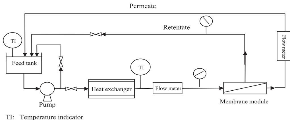
Fig. 1. Schematic diagram of the experimental set-up.
