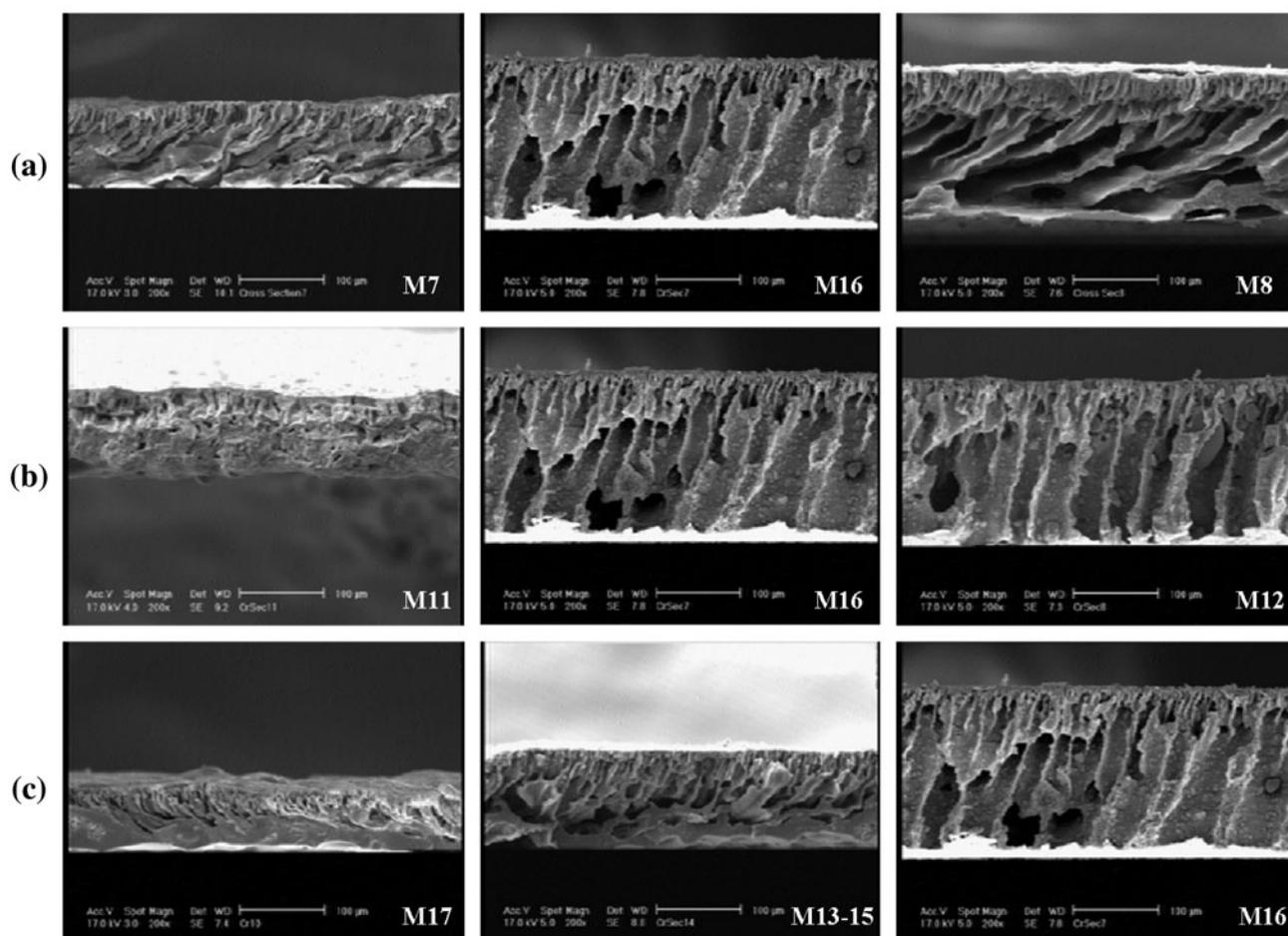
Fig. 2. Effect of CBT (a) starch concentration, (b) sorbitol concentration and (c) on morphology of the synthesized membranes.
