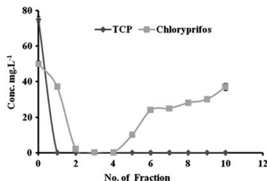
Fig. 5. Filtration of chlorpyrifos and trichloro-2-pyridinol (TCP) by a laboratory filter, which includes a micelle–clay complex mixed with excess sand at 1:50 (w/w). The flow rate was  $2.0 \text{ mL min}^{-1}$ . Initial concentrations of chlorpyrifos and TCP were  $50.0$  and  $75.0 \text{ mg L}^{-1}$ , respectively, pH 6.58, and  $T = 25^\circ\text{C}$ .
