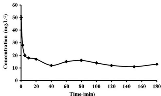
Fig. 3. Percentage removal (%) of chlorpyrifos using micelle–clay complex as a function of time. Initial concentration was  $100 \text{ mg L}^{-1}$ . Adsorbent dose was  $5 \text{ g L}^{-1}$ , pH 6.58, and  $T$   $25^\circ\text{C}$ .
