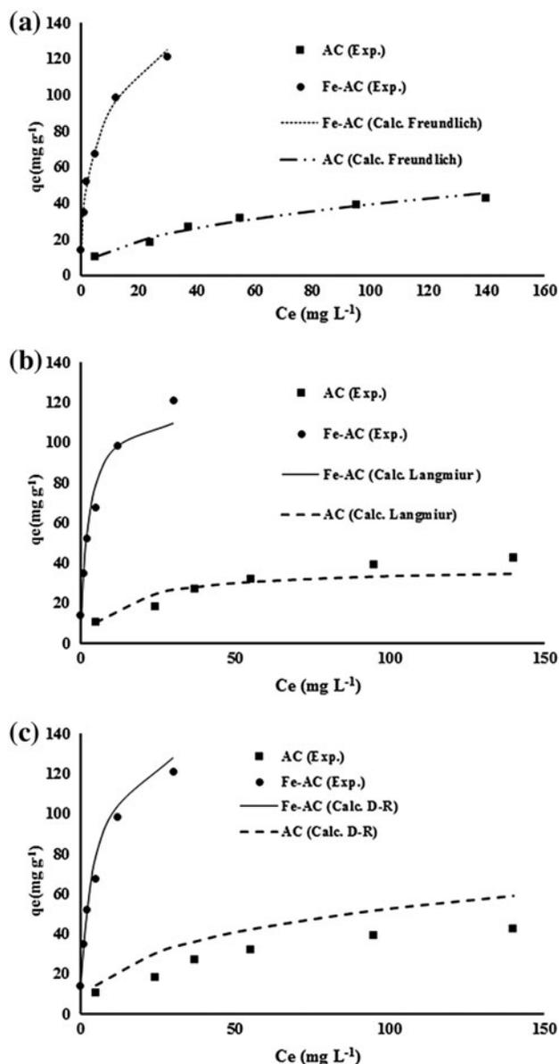
Fig. 7. Equilibrium isotherms of vanadium adsorption on AC and Fe-AC nanocomposites: (a) Freundlich isotherms, (b) Langmuir isotherms, and (c) D-R isotherm.
