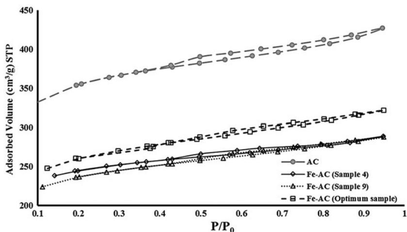
Fig. 6. Adsorption–desorption isotherms of N<sub>2</sub> for adsorbents.
