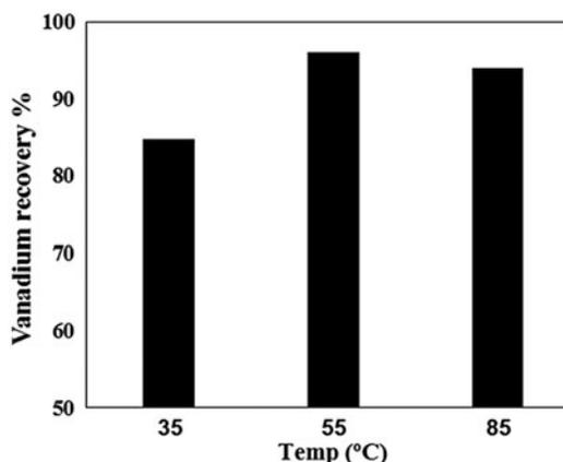
Fig. 3. Effect of temperature (°C) on vanadium recovery by nanoscale Fe-AC nanocomposite.
