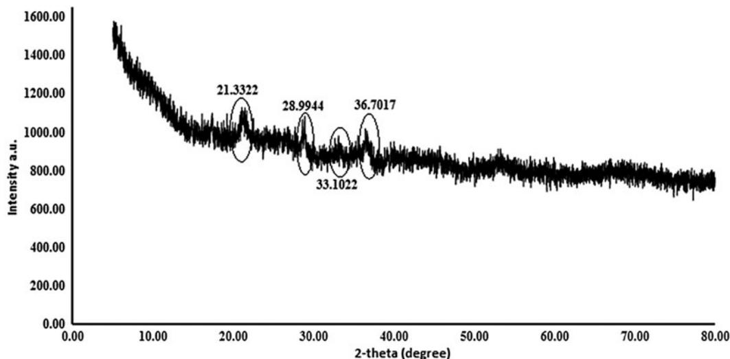
Fig. 4. XRD patterns of Fe-AC nanocomposite.
