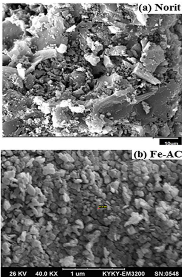
Fig. 5. SEM micrograph of (a) virgin Norit activated carbon and (b) Fe-AC nanocomposite.
