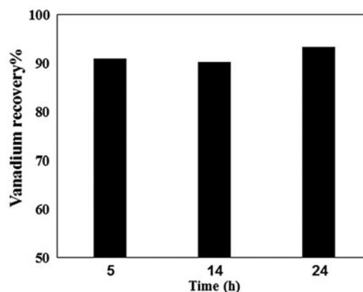
Fig. 2. Effect of contact time (h) on vanadium recovery by nanoscale Fe-AC nanocomposite.
