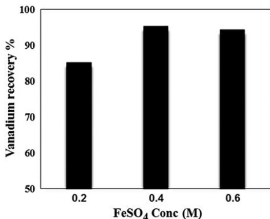
Fig. 1. Effect of FeSO<sub>4</sub> Conc. (M) on vanadium recovery by nanoscale Fe-AC nanocomposite.
