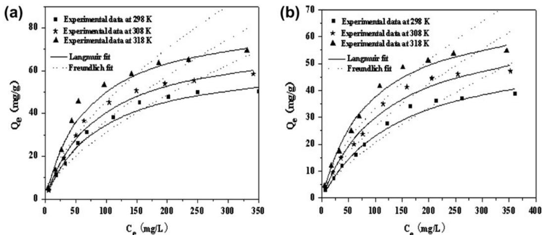
Fig. 6. Comparison of Langmuir and Freundlich isotherm models for 2,4,5-TCP (a) and 2,4,6-TCP (b) adsorption onto  $\beta$ -CD/mATP using nonlinear regression.
