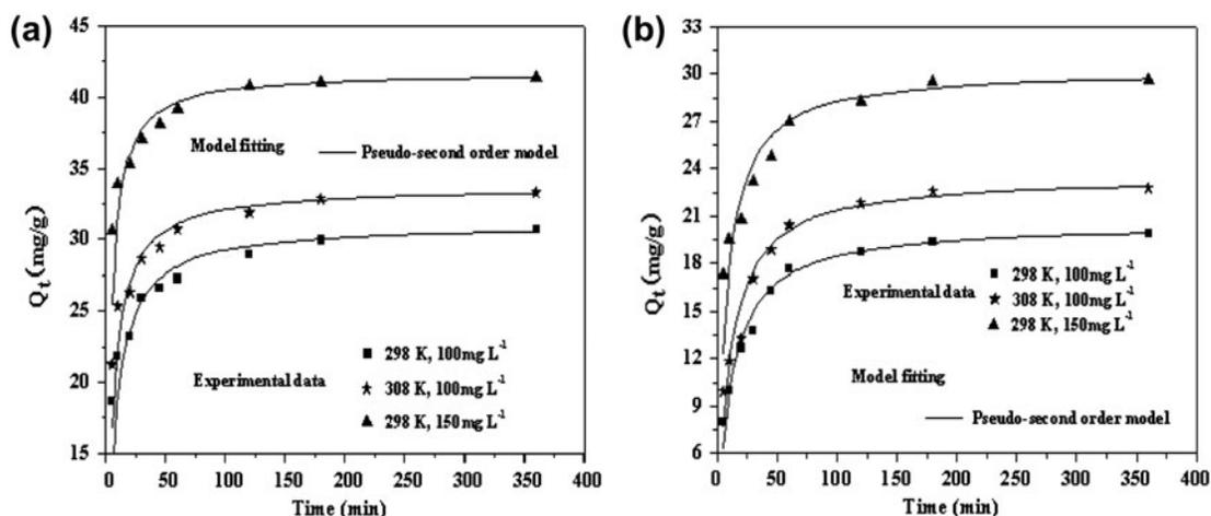
Fig. 5. Kinetic modeling of the effect of initial concentration and temperature for adsorption of 2,4,5-TCP (a) and 2,4,6-TCP (b) onto  $\beta$ -CD/mATP.
