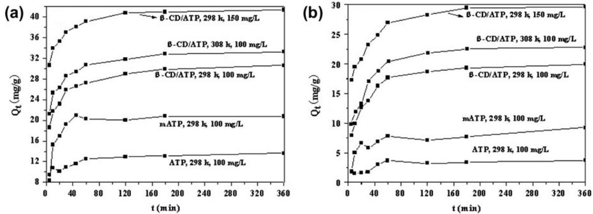
Fig. 4. Effect of contact time at different initial concentrations and temperatures on adsorptive removal of 2,4,5-TCP (a) and 2,4,6-TCP (b).
