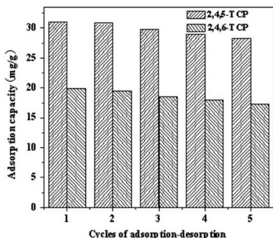
Fig. 7. Adsorption–desorption cycles for  $\beta$ -CD/mATP.
