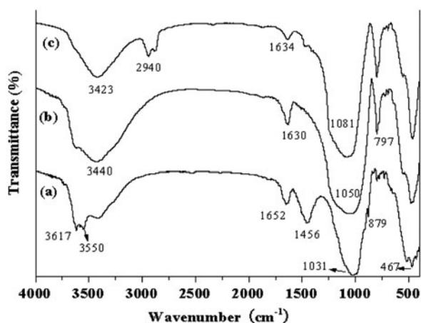
Fig. 2. FT-IR spectra of ATP (a), mATP (b), and  $\beta$ -CD/mATP (c).
