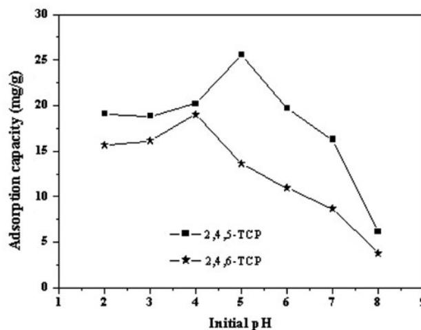
Fig. 3. Effect of pH on adsorptive removal of 2,4,5-TCP and 2,4,6-TCP.
