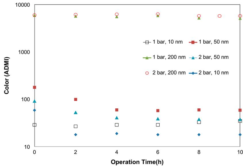
Fig. 3. Impact of membrane pressure and pore size on color removal in the raw water (feed temp:  $20 \pm 2^\circ\text{C}$ , total recycle mode).
