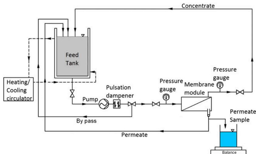
Fig. 1. The schematic diagram of the lab-scale, cross-flow ceramic membrane test unit.
