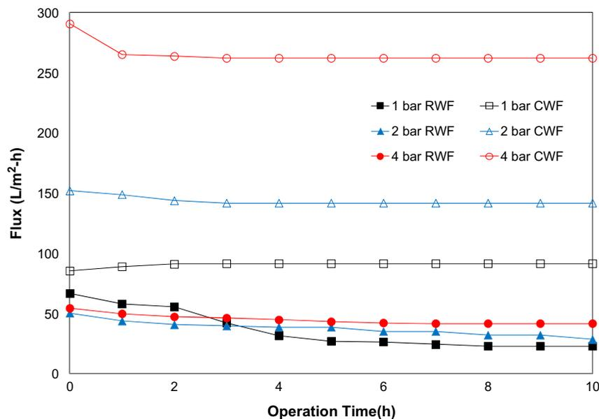
Fig. 2. Impact of membrane pressure on WWF and CFW (membrane average pore size: 10 nm, feed temp:  $20 \pm 2^\circ\text{C}$ , total recycle mode).
