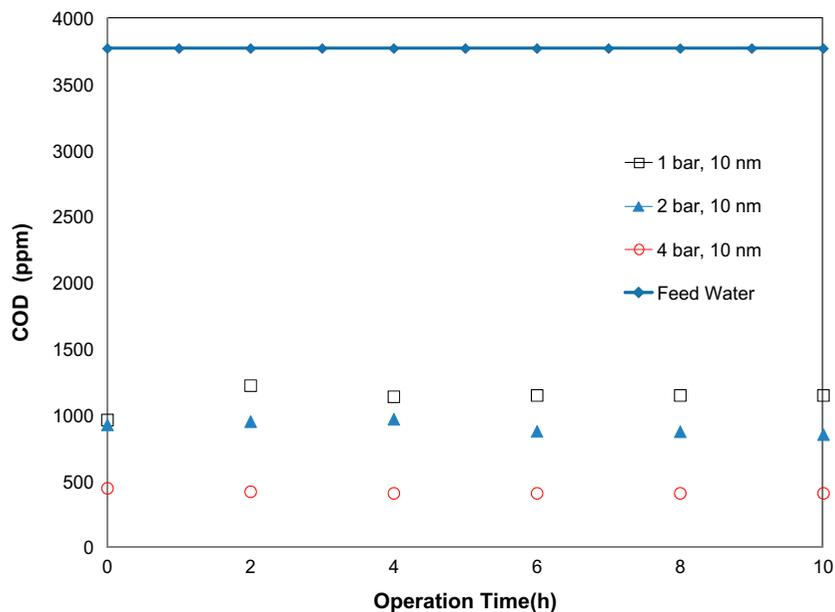
Fig. 5. Impact of membrane pressure on COD removal (pore size: 10 nm, feed flowrate: 2.5 L/min, CFV: 3.3 m/s, feed temp:  $20 \pm 2^\circ\text{C}$ , total recycle mode).
