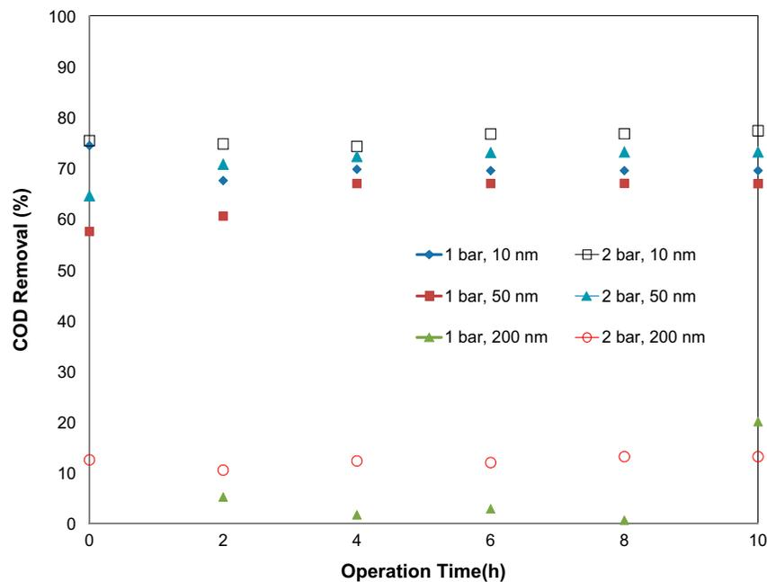
Fig. 4. Impact of membrane pressure and pore size on COD removal in the raw water (feed flowrate: 2.5 L/min, CFV: 3.3 m/s, feed temp:  $20 \pm 2^\circ\text{C}$ , total recycle mode).
