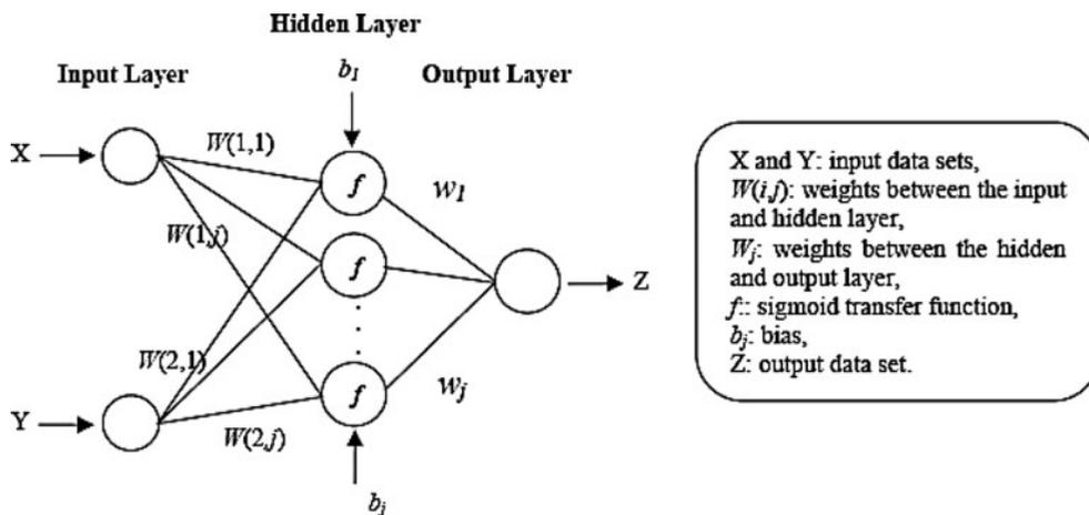
Fig. 3. ANN Architecture for three layers.
