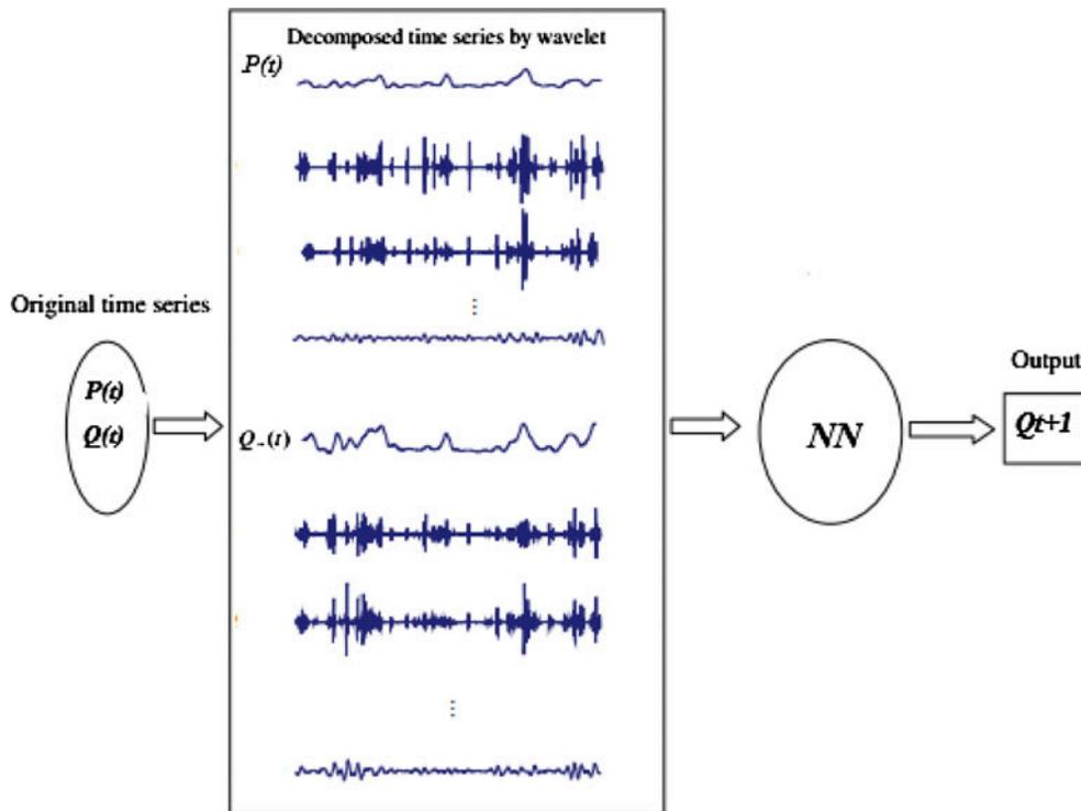
Fig. 5. Structure of the proposed WNN model.
