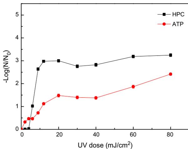
Fig. 3. Disinfection curve of *B. subtilis* by UV. The results were detected by HPC and ATP. Experiment conditions: initial concentration:  $10^6\text{--}10^7$  cells/L; pH 7 with 5 mM phosphate buffer.
