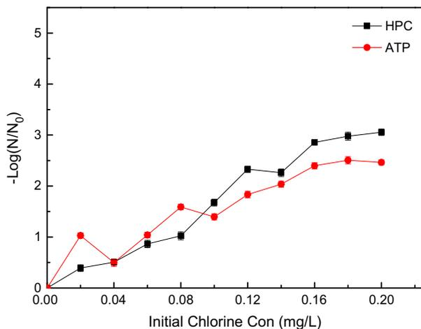
Fig. 7. Disinfection curve of *B. subtilis* by NaClO. The results were detected by HPC and ATP. Experiment conditions:  $10^6$ – $10^7$  cells/L; contact time: 30 min; pH 7 with 5 mM phosphate.
