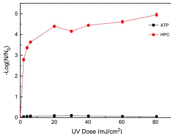
Fig. 1. Disinfection curve of *E. coli* by UV. Detected by HPC and ATP. Experimental conditions: initial concentration:  $10^7$  cells/mL, pH 7 with 5 mM phosphate buffer.
