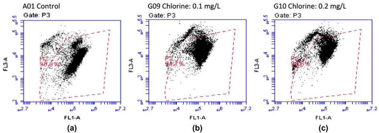
Fig. 6. FCM detection of the membrane integrity of *E. coli* during NaClO disinfection. (a) control, (b) 0.1 mg/L initial chlorine concentration treatment, and (c) 0.2 mg/L initial chlorine concentration treatment.
