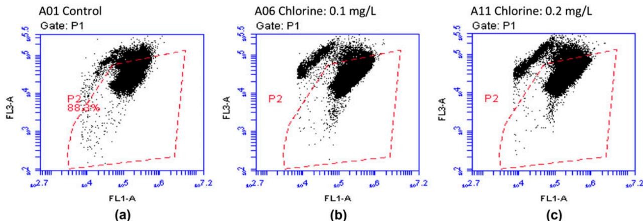
Fig. 8. FCM detection of membrane integrity of *B. subtilis* during chlorine disinfection. (a) control, (b) 0.1 mg/L initial chlorine concentration treatment, and (c) 0.2 mg/L initial chlorine concentration treatment.
