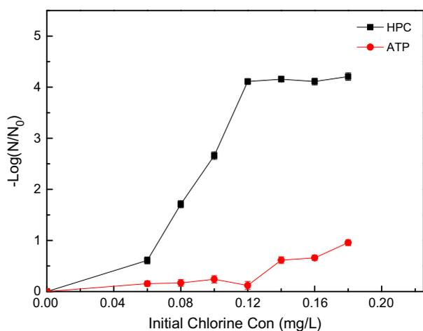
Fig. 5. Disinfection curve of *E. coli* by NaClO. The results were detected by HPC and ATP. Experiment conditions: initial concentration: 10<sup>7</sup> cells/L, contact time: 30 min, pH 7 with 5 mM phosphate buffer.
