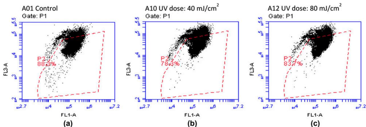
Fig. 4. FCM detection of membrane integrity of *B. subtilis* during UV disinfection. (a) control, (b) 40 mJ/cm<sup>2</sup> treatment, and (c) 80 mJ/cm<sup>2</sup> treatment.
