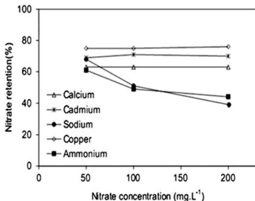
Fig. 18. Evolution of the rejection rate of  $\text{NO}_3^-$  as function of  $C_i$  for different salts.
