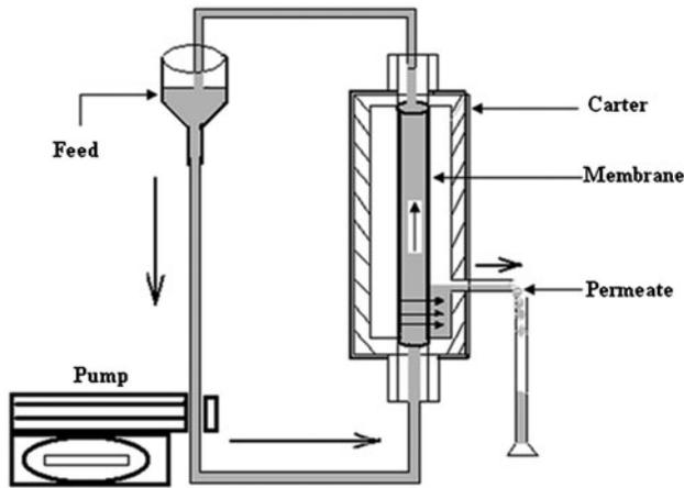
Fig. 5. Schematic of the pilot system.
