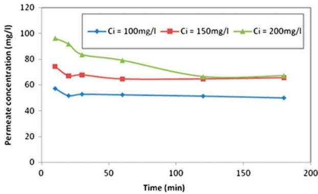
Fig. 15. Retention of  $\text{NO}_3^-$  as a function of time and concentration.
