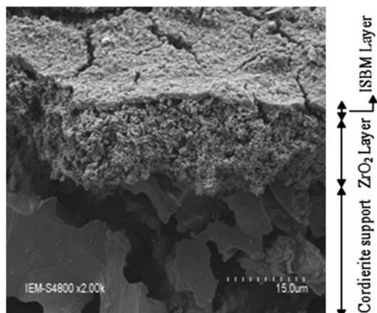
Fig. 11. Scanning electron micrographs of cordierite/ZrO<sub>2</sub>/ISBMA membrane.
