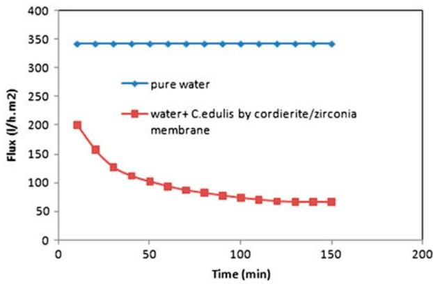
Fig. 4. Variation of flow of distilled water + ISBMA as a function of filtration time.
