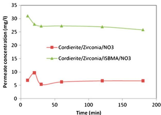
Fig. 13. Permeate concentration of  $\text{NO}_3^-$  as a function of time.
