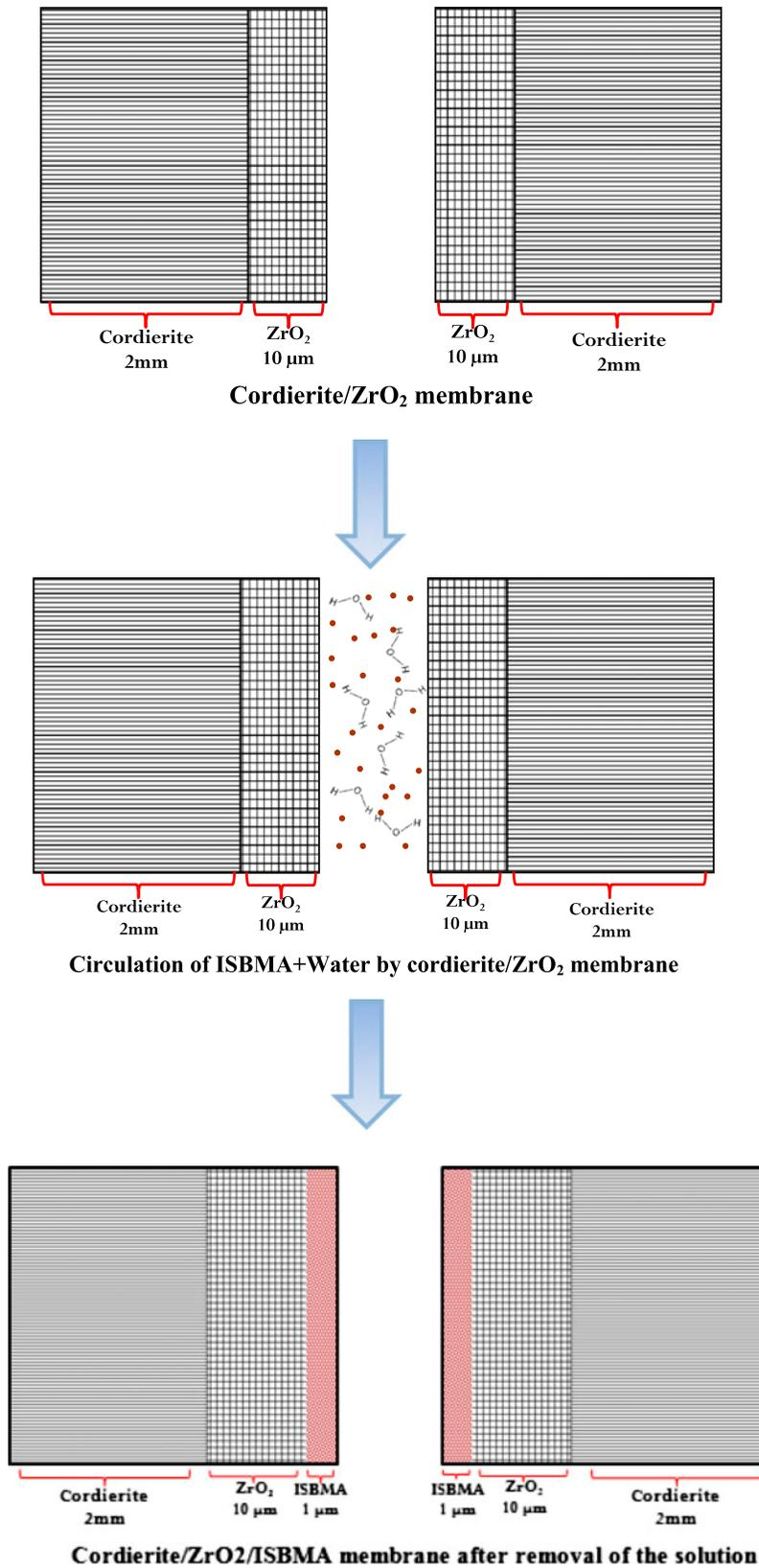
Fig. 3. Cordierite/ZrO<sub>2</sub>/ISBMA membrane preparation.
