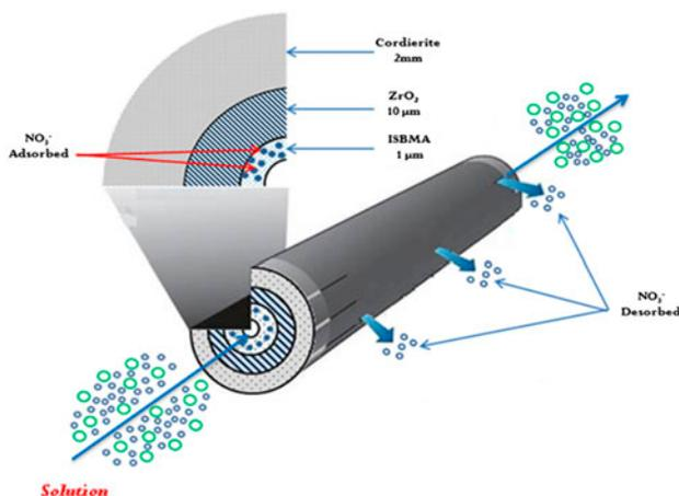
Fig. 12. Rejection of  $\text{NO}_3^-$  by cordierite/ $\text{ZrO}_2$ /ISBMA membrane.
