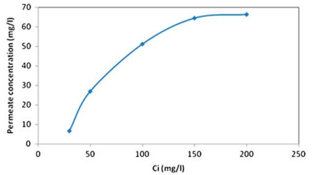
Fig. 17. Retention of  $\text{NO}_3^-$  as a function of concentration.
