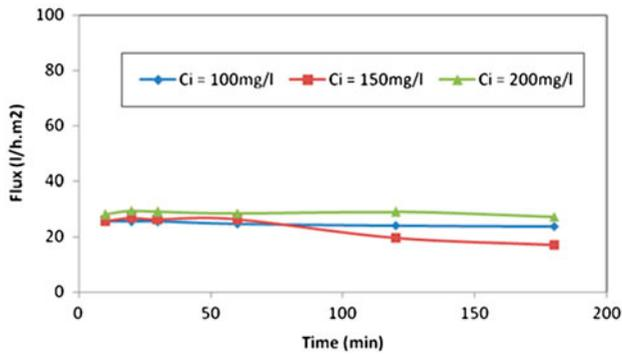
Fig. 14. Variation of flux of  $\text{NO}_3^-$  as a function of time and concentration.
