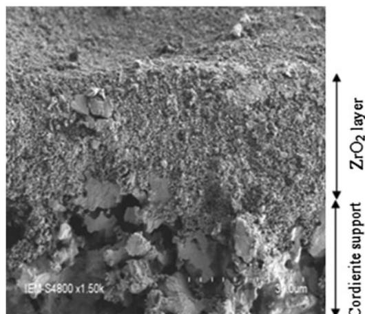
Fig. 10. Scanning electron micrographs of cordierite/ZrO<sub>2</sub> membrane.
