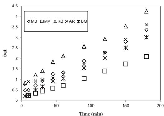
Fig. 6. Second-order kinetic equation for the adsorption of dyes on CSAC at 100 mg/L initial dye concentration.
