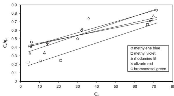
Fig. 7. Langmuir adsorption isotherm plots for the adsorption of dyes at 30°C.
