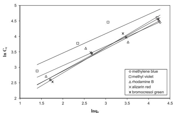
Fig. 8. Freundlich adsorption isotherm plots for the adsorption of dyes at 30°C.
