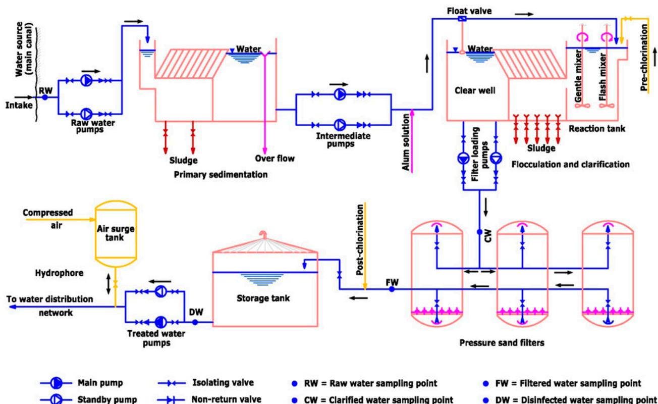
Fig. 1. A schematic flow diagram of the processes within the HC-DWTP of Assiut University.
