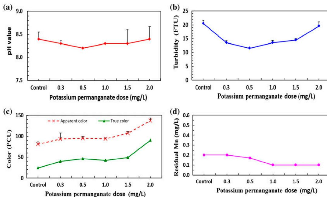
Fig. 5. Jar test results for the effects of permanganate pretreatment doses on the water characters of the enriched water sample; (a) pH value, (b) turbidity, (c) apparent and true colors, and (d) residual manganese (Mn). The error bars indicate standard errors. The data represent the means  $\pm$  SE,  $n = 3$ .
