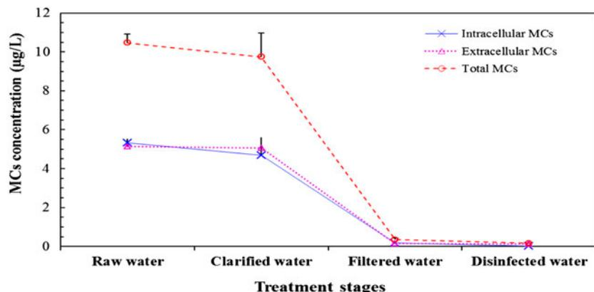
Fig. 4. The measured MCs concentration within the full-scale plant through the treatment line, without pre-chlorination. The error bars indicate standard errors. The data represent the means  $\pm$  SE,  $n = 2$ .
