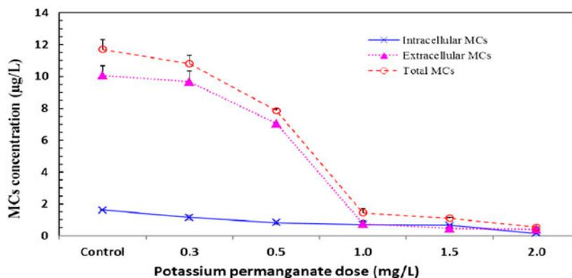
Fig. 6. Jar test results for the effect of permanganate pretreatment doses on the measured MCs concentration of the enriched water sample. The error bars indicate standard errors. The data represent the means  $\pm$  SE,  $n = 2$ .
