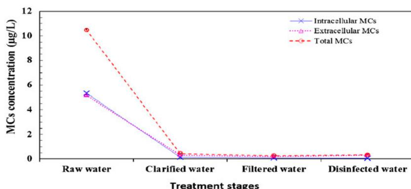
Fig. 3. The measured MCs concentration within the full-scale plant through the treatment line, with pre-chlorination. The error bars indicate standard errors. The data represent the means  $\pm$  SE,  $n = 2$ .
