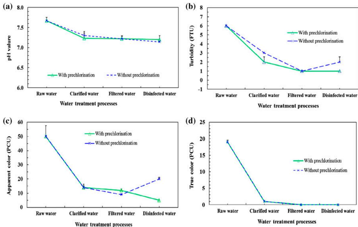
Fig. 2. The measured characteristics of the water through two treatment scenarios within the full-scale plant, with and without pre-chlorination; (a) pH value, (b) turbidity, (c) apparent color, and (d) true color. The error bars indicate standard errors. The data represent the means  $\pm$  SE,  $n = 3$ .
