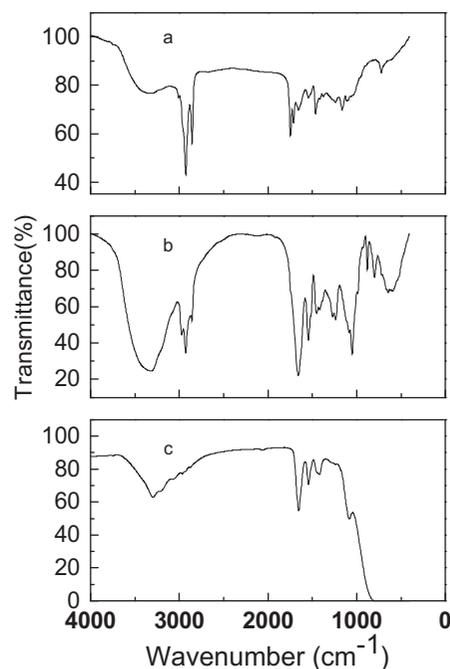
Fig. 1. FTIR spectrum of MOSCP (a), MOSCP-AEP (b), and MOSCP-E (c).
