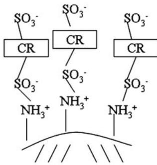
Fig. 3. Schematic illustration of the coagulation mechanism of CR dye with MOSCP.
