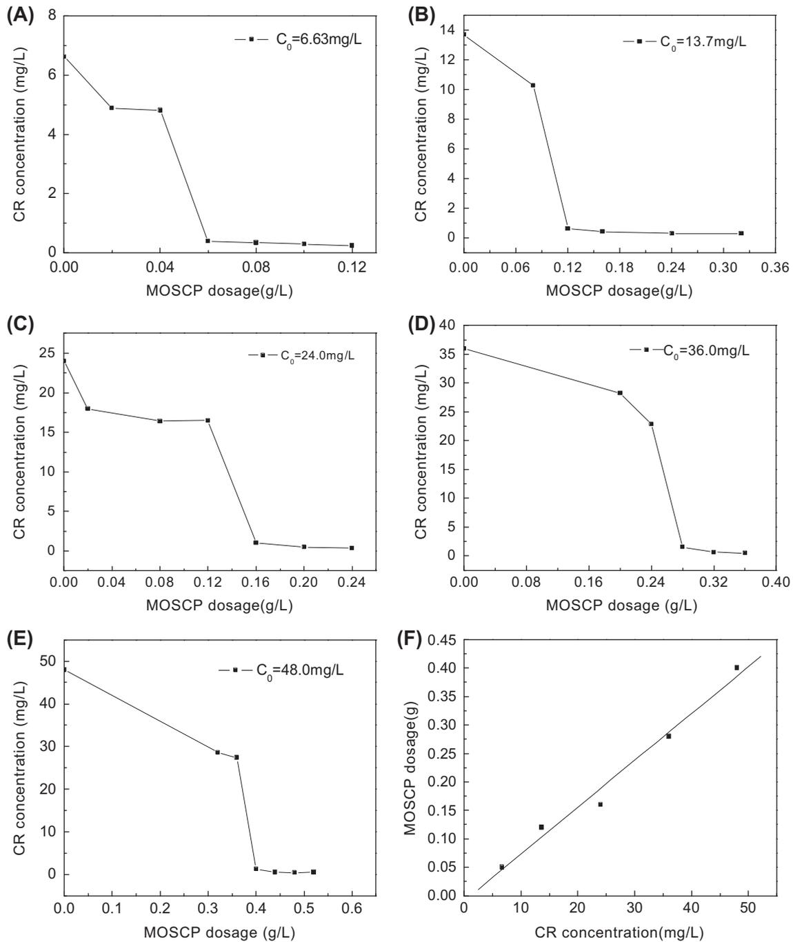
Fig. 5. Effect of MOSCP dosage and CR concentration on CR removal (A–E) and the relationship between CR concentration and saturated MOSCP dosage (F) ( $T = 21 \pm 2^\circ\text{C}$ , settling time = 0.5 h).
