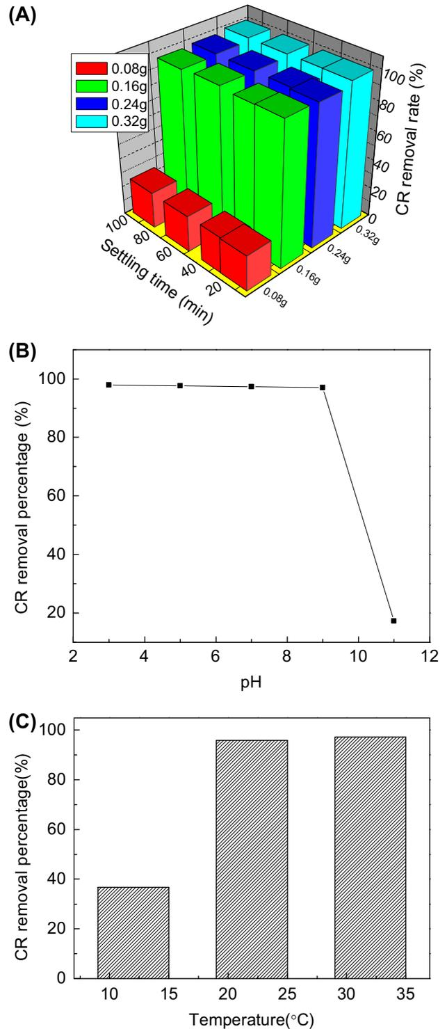
Fig. 4. Effect of settling time (A), pH (B), and temperature (C) on CR removal (A:  $C_0 = 13.7 \text{ mg/L}$ ,  $T = 21 \pm 2^\circ\text{C}$ ; B:  $T = 21 \pm 2^\circ\text{C}$ ,  $C_0 = 24 \text{ mg/L}$ , MOSCP:  $0.16 \text{ g/L}$ , settling time =  $0.5 \text{ h}$ ; C:  $C_0 = 24 \text{ mg/L}$ , MOSCP:  $0.16 \text{ g/L}$ , settling time =  $0.5 \text{ h}$ ).
