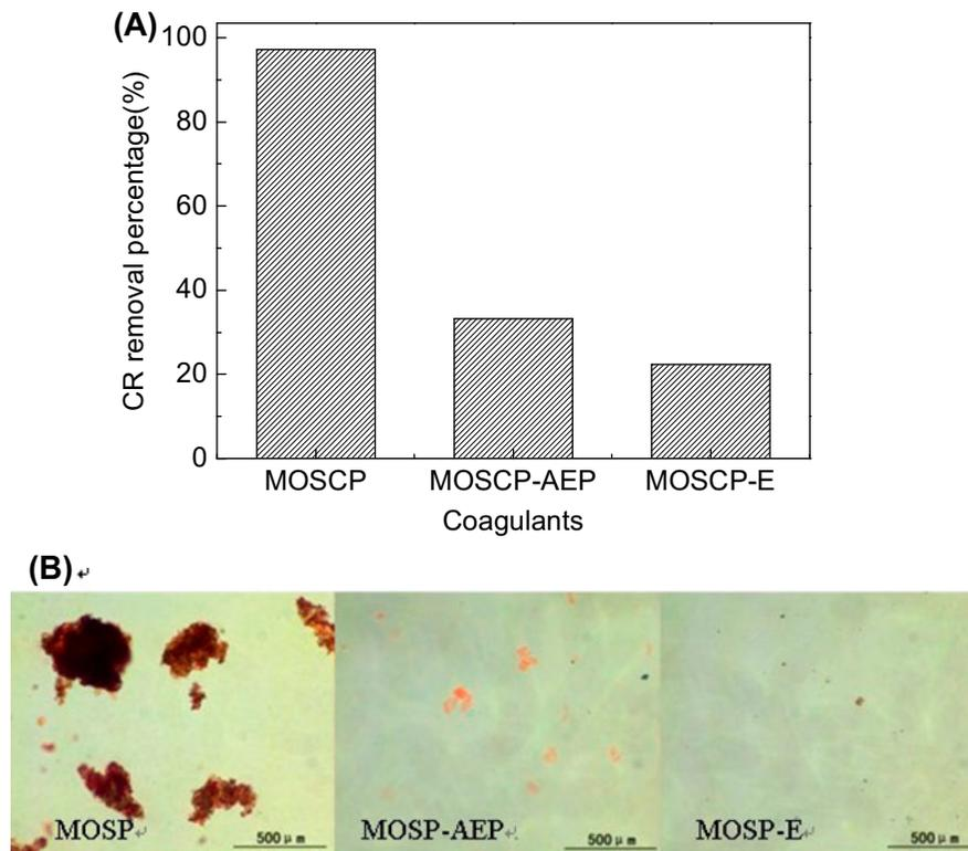
Fig. 2. Effect of three coagulants on CR removal (A) and the microscope photographs of flocs formed by the coagulants (B) (coagulant dosage: MOSCP: 0.16 g/L, MOSCP-AEP: 0.16 g/L, MOSCP-E: 8 ml (equals to 0.16 g/L MOSCP),  $T = 30 \pm 2^\circ\text{C}$ , settling time = 0.5 h,  $C_0 = 24 \text{ mg/L}$ ).
