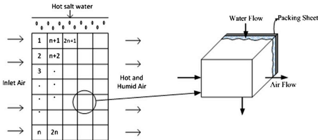
Fig. 2. Grid elements of packing in humidifier.
