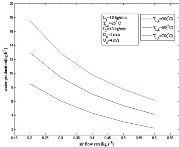
Fig. 9. Condensation rate vs. air flow rate.
