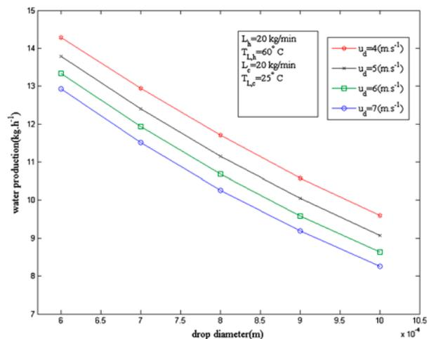
Fig. 5. Effect of inlet water droplets diameter to dehumidifier on fresh water production.
