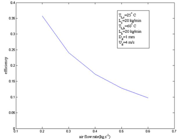
Fig. 14. Efficiency vs. air mass flow rate.
