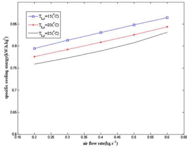
Fig. 12. Specific cooling energy vs. air flow rate.
