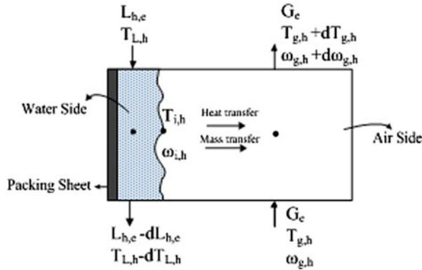
Fig. 3. One element of humidifier and heat and mass transfer direction.
