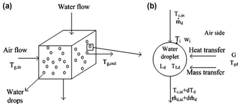
Fig. 4. (a) One element of dehumidifier and (b) heat and mass transfer direction.
