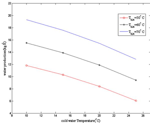
Fig. 6. Effect of inlet water temperature to dehumidifier on fresh water production.
