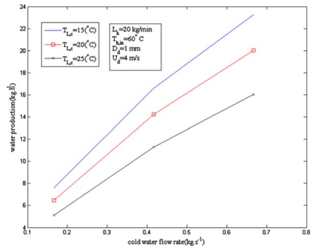
Fig. 7. Effect of inlet water flow rate to dehumidifier on fresh water production.
