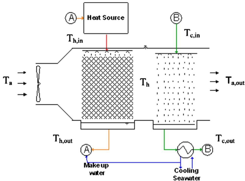
Fig. 1. Sketch of the HD unit with an opened air cycle and water heating.
