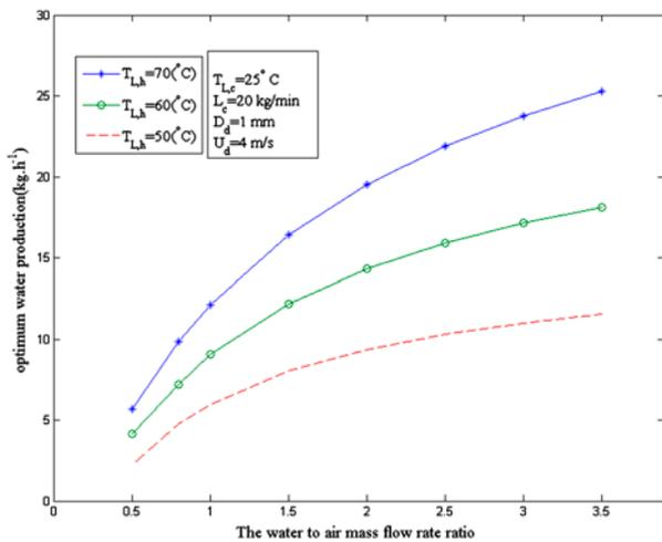
Fig. 10. Optimum water production vs. L<sub>h</sub>/G.
