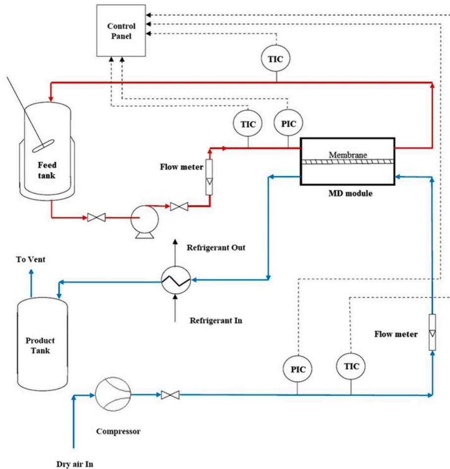
Fig. 1. The general scheme of the experimental setup.
