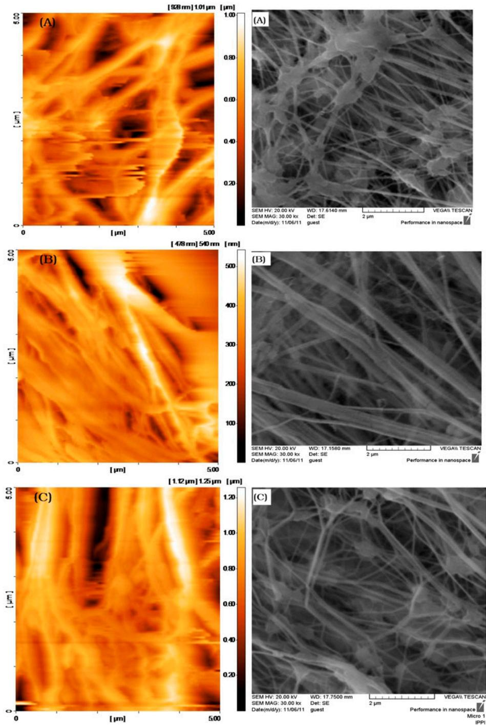
Fig. 2. AFM (left) and SEM (right) images of the investigated PTFE membranes, (A) M1, (B) M2, and (C) M3, respectively.
