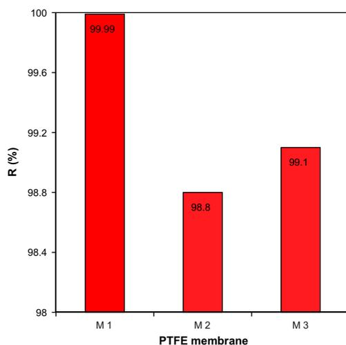
Fig. 4. Solute-rejection evaluation of the applied PTFE membranes (65°C feed temperature, 600 mL/min feed flow rate, and 0.453 Nm<sup>3</sup>/h sweeping gas flow rate).
