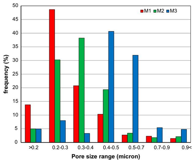
Fig. 3. Pore size distribution of applied membranes based on the AFM analysis (M1, M2, and M3).
