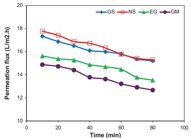
Fig. 5. Permeation flux for various feed samples versus operating time (65°C feed temperature, 600 mL/min feed flow rate, and 0.453 Nm<sup>3</sup>/h sweeping gas flow rate).
