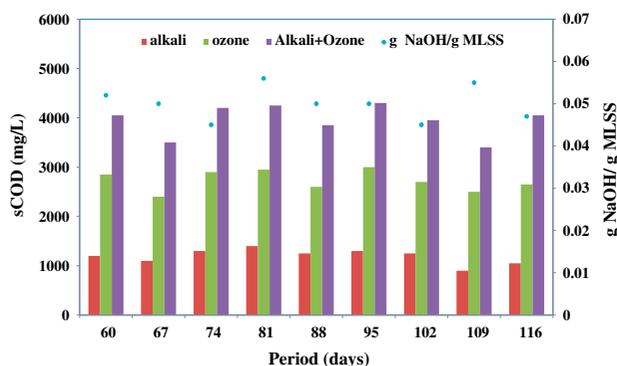
Fig. 3. Effect of alkali-ozone pretreatment on SCOD release during the study period.
