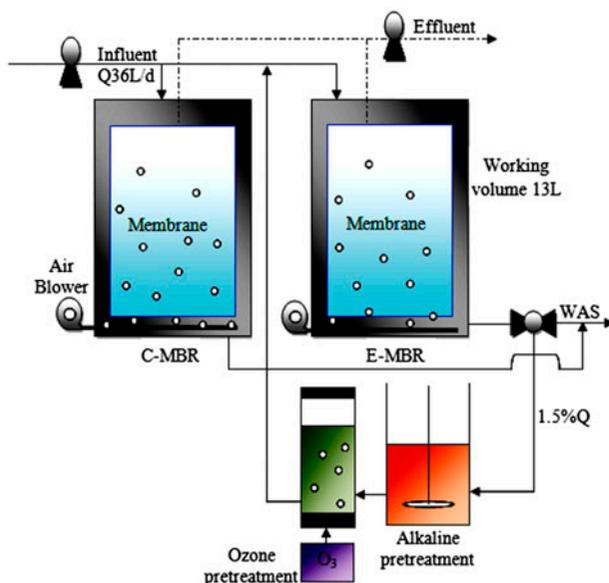
Fig. 1. Schematic representation of MBR with (EMBR) and without (CMBR) sludge pretreatment.
