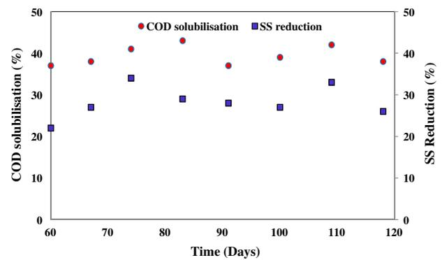
Fig. 4. Effect of alkali-ozone pretreatment on COD solubilization and SS reduction.
