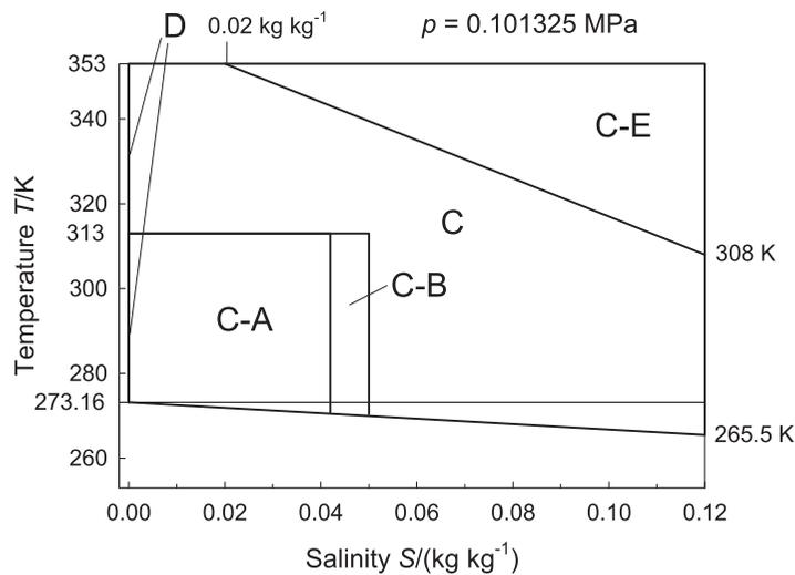
Fig. 2.  $T$ - $S$  diagram of seawater at standard atmospheric pressure  $p_0 = 0.101325 \text{ MPa}$  with the regions C and D of the  $T$ - $S$  plane and the intersections of the regions A, B, and E with region C (C-A, C-B, C-E).
