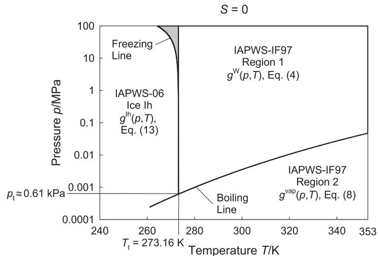
Fig. 6.  $p$ - $T$  diagram of pure water (salinity  $S = 0$ ) showing the Gibbs equations of Region 1 (liquid) and Region 2 (vapor) of IAPWS-IF97 as well as the Gibbs equation of the ice Ih region of IAPWS-06. In the gray-shaded area, the Gibbs equation of IAPWS-IF97 Region 1 is extrapolated to temperatures below its range of validity in the metastable region.
