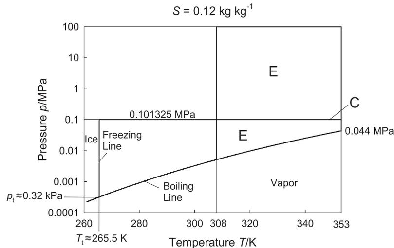
Fig. 5.  $p$ - $T$  diagram of seawater at salinity  $S = 0.12 \text{ kg kg}^{-1}$  with the regions C and E of the  $p$ - $T$  plane.
