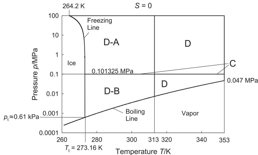
Fig. 3.  $p$ - $T$  diagram of seawater at salinity  $S=0$  (pure water) with the regions C and D of the  $p$ - $T$  plane and the intersections of the regions A and B with region D (D-A, D-B).
