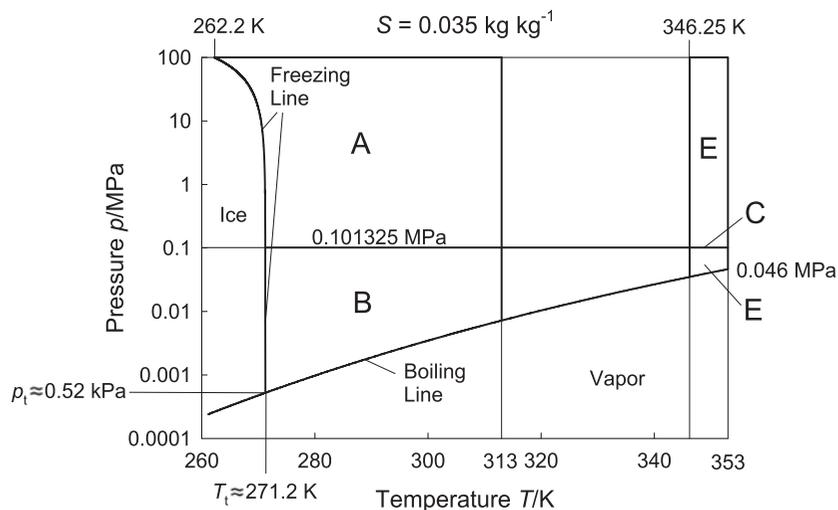
Fig. 4.  $p$ - $T$  diagram of seawater at salinity  $S = 0.035 \text{kg kg}^{-1}$  with the regions A, B, C, and E of the  $p$ - $T$  plane.
