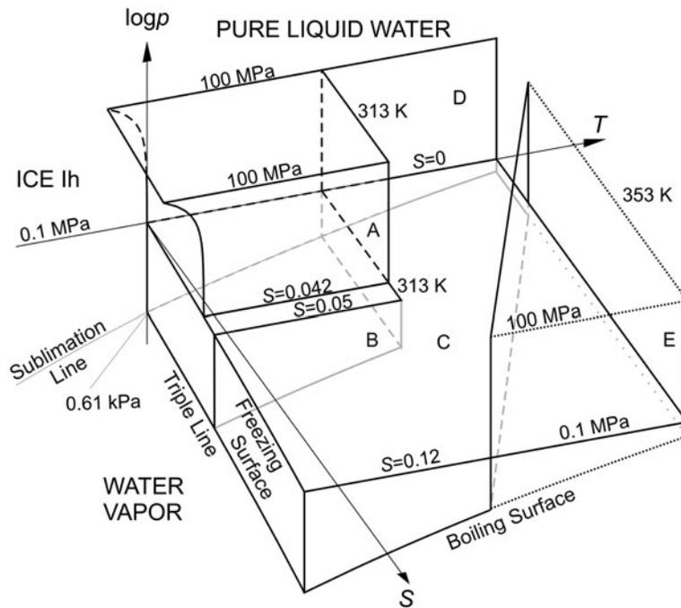
Fig. 1. Phase diagram of seawater with the regions A to E of  $p$ - $T$ - $S$  space (values of salinity  $S$  in  $\text{kg kg}^{-1}$ ). Regions A, B, and E are three-dimensional volumes. Region C is planar at  $p = 0.1 \text{ MPa}$ , region D is planar at  $S = 0$ . The intersection of the boiling surface with the plane  $S = 0$  is the saturation curve of pure water (not indicated in the graph).
