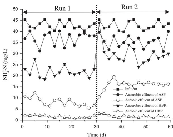
Fig. 3. The influent and effluent NH<sub>4</sub><sup>+</sup>-N concentrations of the two processes during continuous operation. Run 1: the loads are 0.97 kg COD<sub>Cr</sub>/m<sup>3</sup>d; Run 2: the loads are 1.94 kg COD<sub>Cr</sub>/m<sup>3</sup>d.
