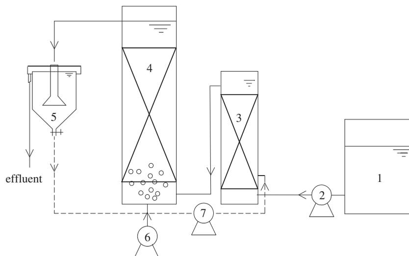
Fig. 1. Experimental set-up and flow chart: (1) storage tank; (2) metering pump for inlet; (3) anaerobic column; (4) aerobic column; (5) settled tank; (6) air pump; and (7) pump for return mixed liquor.
