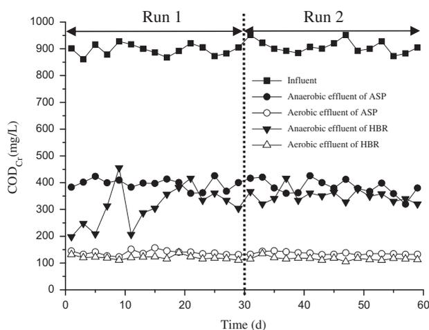
Fig. 2. The influent and effluent  $COD_{Cr}$  concentrations of the two processes during continuous operation. Run 1: the loads are  $0.97 \text{ kg } COD_{Cr}/\text{m}^3 \text{ d}$ ; Run 2: the loads are  $1.94 \text{ kg } COD_{Cr}/\text{m}^3 \text{ d}$ .
