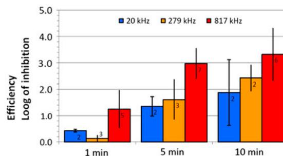
Fig. 6. Inhibition of *E. coli* as a function of treatment time.
