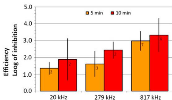
Fig. 5. Inhibition of *E. coli* as a function of applied frequency.
