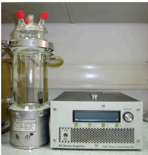
Fig. 2. High-frequency (279/817 kHz) plate ultrasound system.
