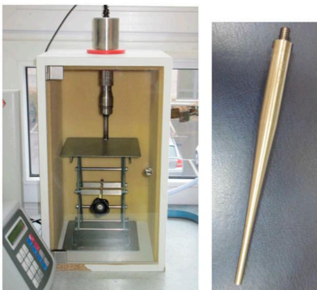
Fig. 1. 20 kHz probe ultrasound system with replaceable tip (left) and tapered micro-tip (right).
