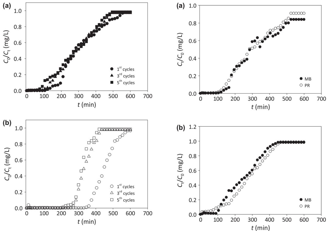
Fig. 6. Regeneration of CA-EFB and PEI-EFB for five adsorption/desorption cycles: (a) MB in a fixed-bed CA-EFB and (b) PR in a fixed-bed PEI-EFB (total adsorbate dose: 300 mg/L; total bed height: 5 cm; temperature: 20°C; and flow rate: 15 mL/min).
