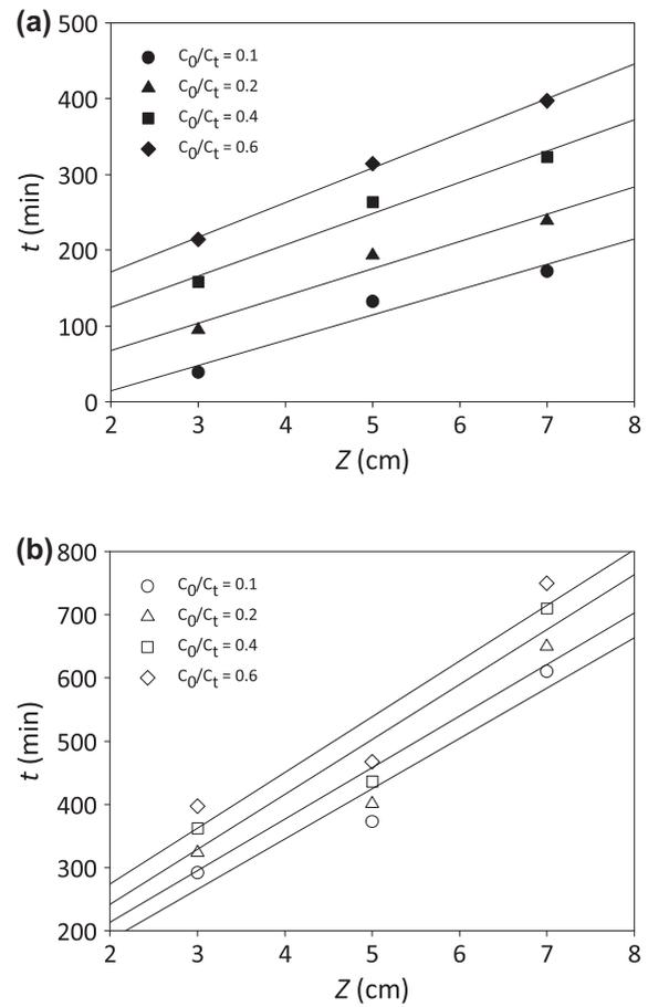
Fig. 5. Linearized plots of BDST model: (a) adsorption of MB by a fixed-bed CA-EFB and (b) adsorption of PR by a fixed-bed PEI-EFB (adsorbate dose: 300 mg/L; bed height: 5–9 cm; temperature: 20–60 °C; and flow rate: 15 mL/min).
