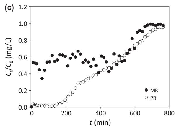
Fig. 7. Adsorption of mixed dyes (MB and PR) using a fixed-bed column with different adsorbent configurations: (a) CA-EFB:PEI-EFB, (b) PEI-EFB:CA-EFB, and (c) mixed CA/PEI-EFB fibers (total adsorbate dose: 300 mg/L; total bed height: 5 cm; temperature: 20°C; pH: 5; and flow rate: 15 mL/min).
