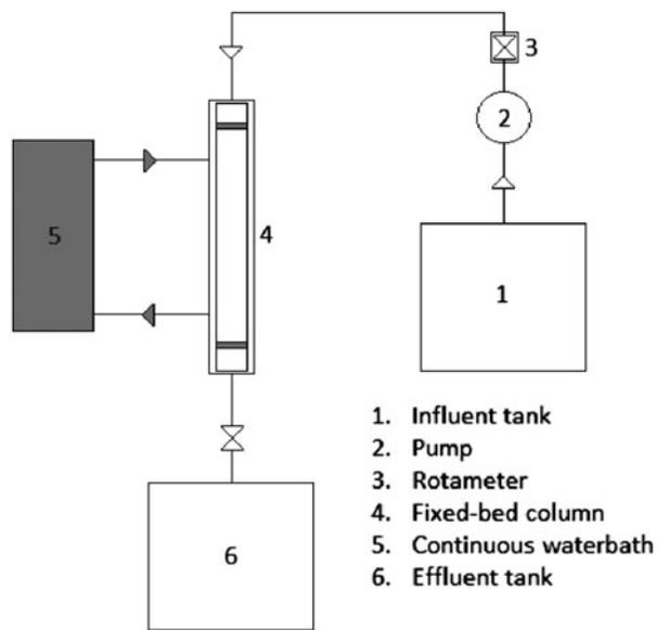
Fig. 2. Schematic diagram of the fixed-bed adsorption system.
