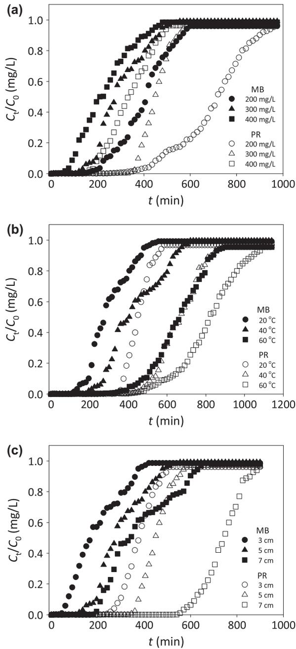
Fig. 4. Adsorption of MB and PR using a fixed-bed CA-EFB and PEI-EFB column, respectively, with different controlled parameters: (a) different initial influent concentrations, (b) different column temperatures, and (c) different column bed heights (adsorbate dose: 200–400 mg/L; bed height: 5–9 cm; temperature: 20–60 °C; and flow rate: 15 mL/min).
