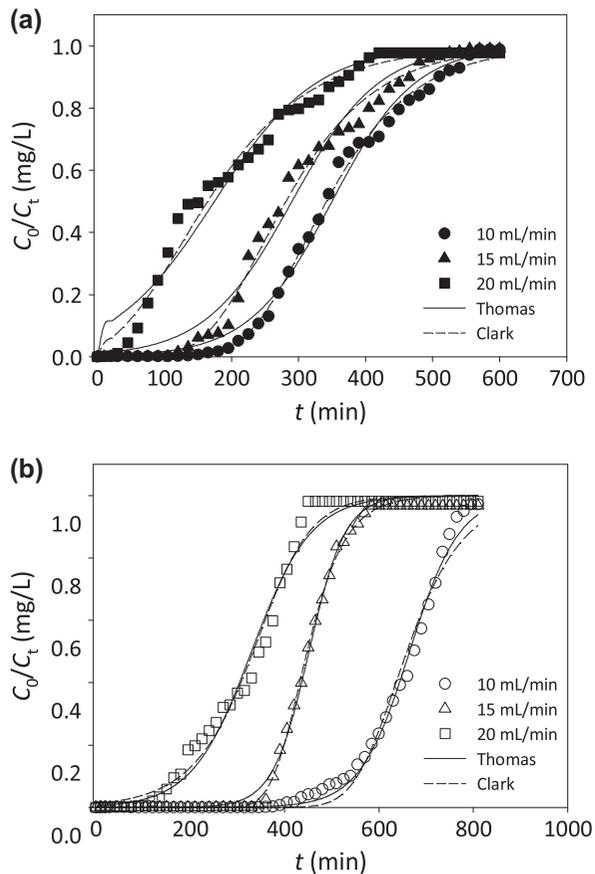
Fig. 3. Non-linearized estimation fits obtained using Thomas and Clark models at different flow rates: (a) MB with a fixed-bed CA-EFB and (b) PR with PEI-EFB (adsorbate dose: 300 mg/L; bed height: 5 cm; temperature: 20°C; and flow rate: 10–20 mL/min).
