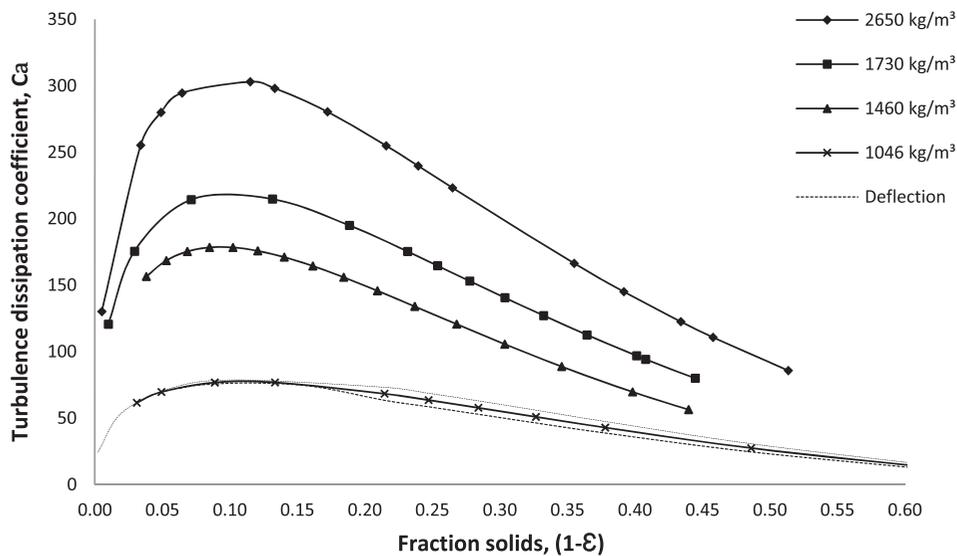
Fig. 10. Turbulence dissipation coefficient vs fraction solids.
