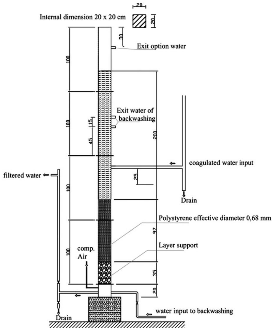
Fig. 6. Scheme of the pilot filter with PS granules as filter element (cm).
