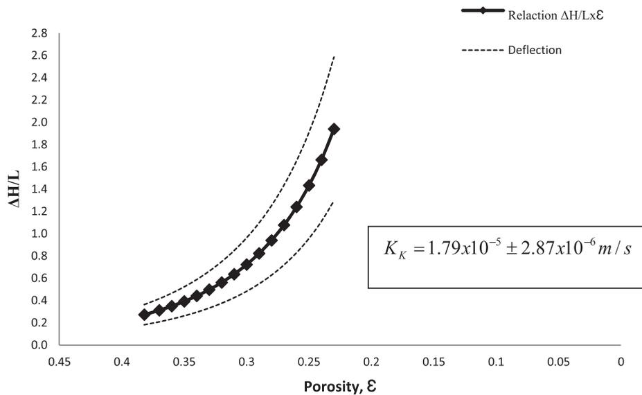
Fig. 12. Curve  $\Delta H/L$  on different stages of clogging of the filter according to the permeability coefficient.
