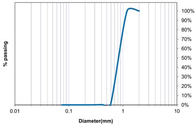
Fig. 2. Granulometric curve PS.
