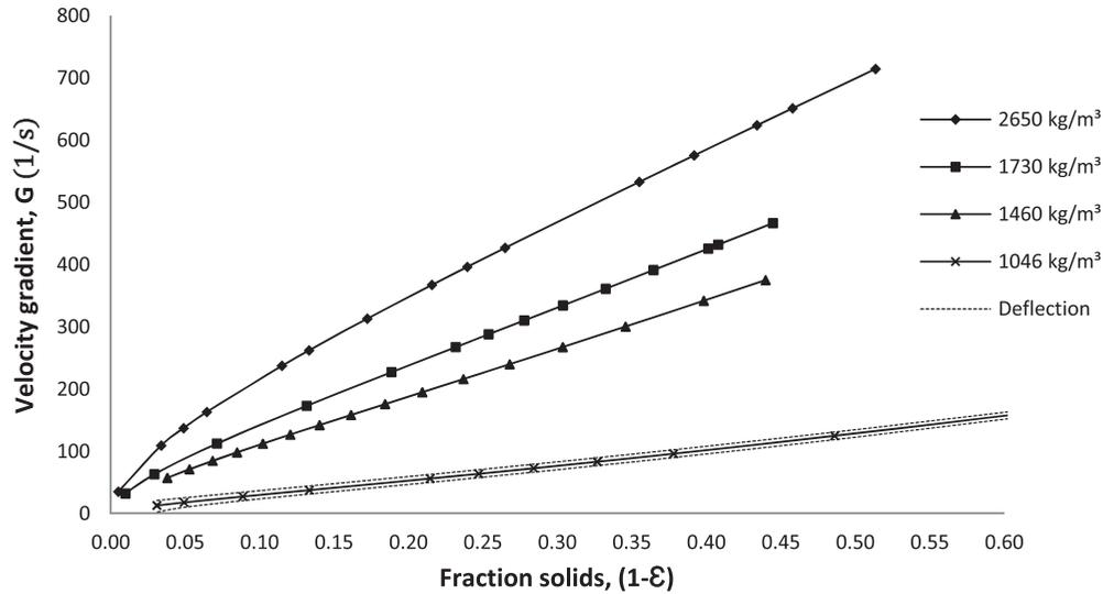
Fig. 9. Velocity gradient vs fraction solids.
