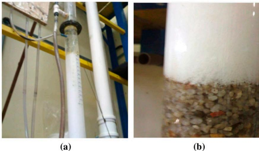
Fig. 3. (a) Acrylic column and level chamber built with level markers that indicate head loss during the expansion test (b) the support layer of the material under analysis.
