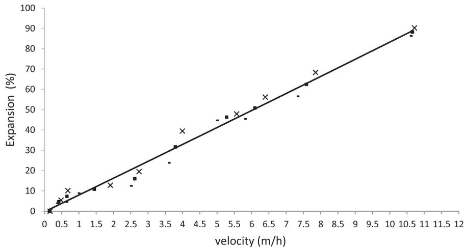
Fig. 5. PS expansion test (Expansion (%) x velocity (m/h)).
