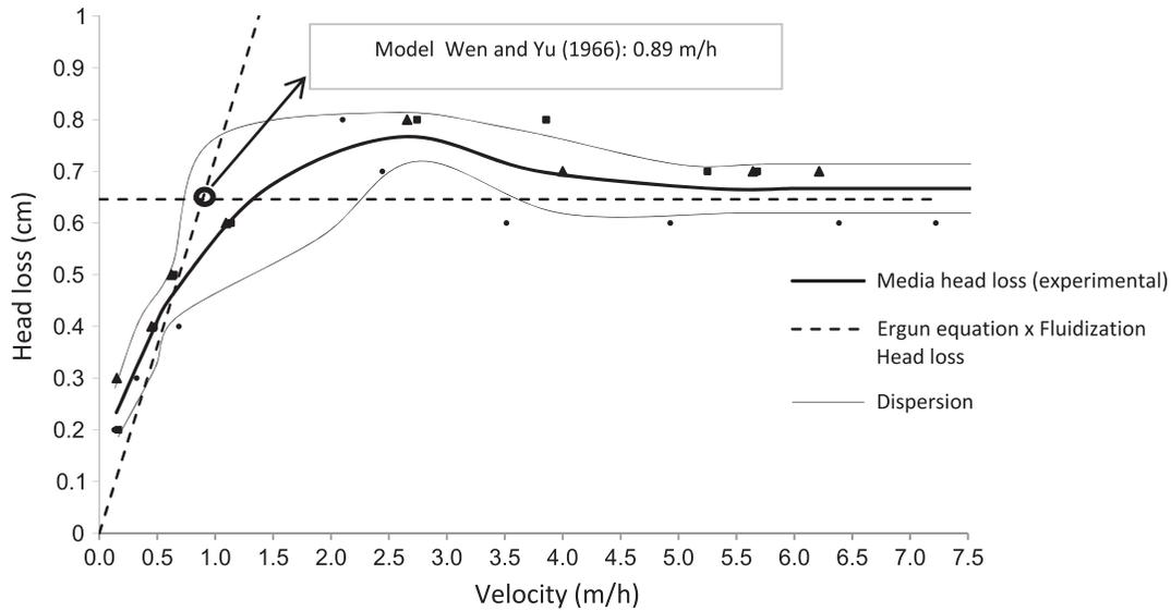
Fig. 4. Experimental results of the head loss curve according to fluidization velocity by the Wen and Yu model [6].
