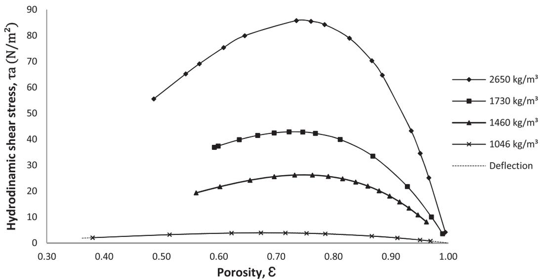
Fig. 8. Hydrodynamic shear-stress variation as a function of porosity for different media filters.
