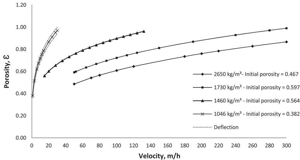
Fig. 7. The porosity calculated of the expanded bed vs superficial velocity of materials with different specific densities.
