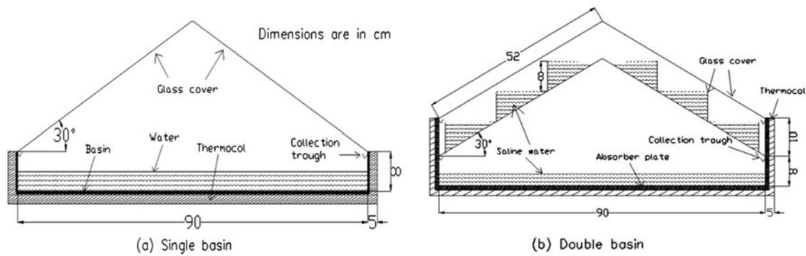
Fig. 1. Schematic view of solar stills.
