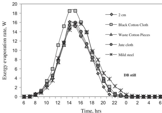
Fig. 9. Variation of exergy evaporation rate for different materials in double-basin still.
