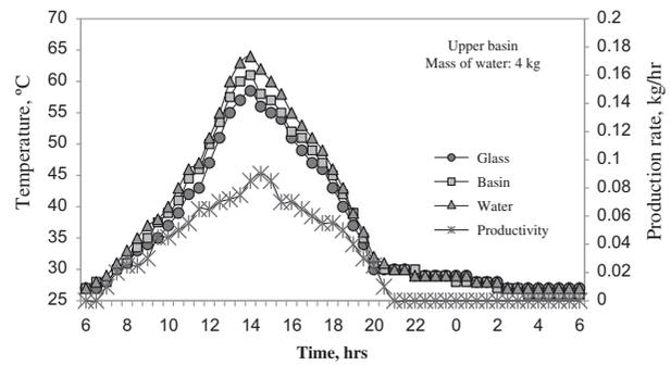
Fig. 5. Variation of different parameters in upper basin of double-basin solar still.
