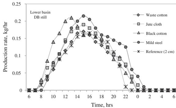
Fig. 7. Variation of lower basin productivity with different materials in basin.
