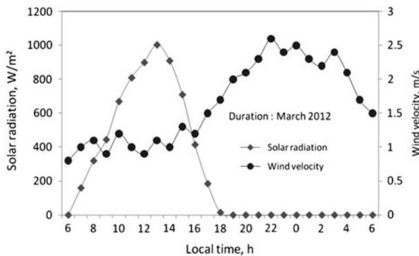
Fig. 4. Variation of solar radiation and wind velocity.
