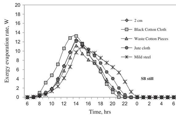
Fig. 10. Variation of exergy evaporation rate for different materials in single-basin still.
