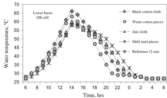
Fig. 6. Variation of lower basin water temperature with different materials in basin.
