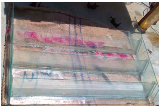
Fig. 3. Photographic view of the upper basin of the double-basin still.
