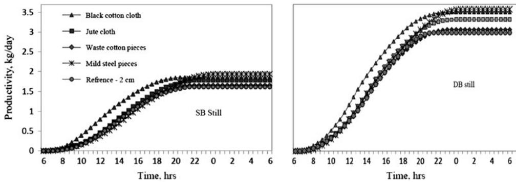
Fig. 8. Variation of cumulative productivity of the single- and double-basin stills.
