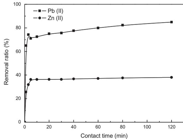
Fig. 3. Effect of contact time on removal of Pb(II) and Zn (II) (conditions: initial metal concentration 20 mg L<sup>-1</sup>, temperature 25 °C, pH 5 and biomass dosage 1.0 g L<sup>-1</sup>).
