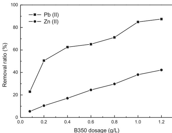
Fig. 2. Effect of B350 dosage on removal of Pb(II) and Zn (II) (conditions: initial metal concentration 20 mg L<sup>-1</sup>, temperature 25 °C, pH 5 and contact time 2 h).
