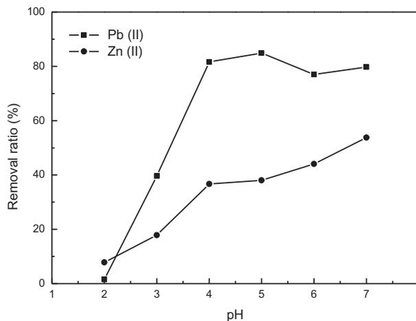
Fig. 1. Effect of pH on removal of Pb(II) and Zn(II) (conditions: initial metal concentration  $20 \text{ mg L}^{-1}$ , temperature  $25^\circ\text{C}$ , contact time 2 h and biomass dosage  $1.0 \text{ g L}^{-1}$ ).
