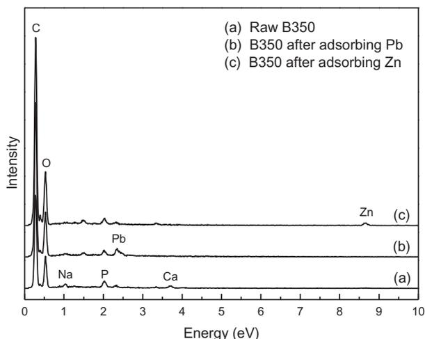
Fig. 4. EDX spectra of B350 before and after adsorbing Pb (II) and Zn(II).
