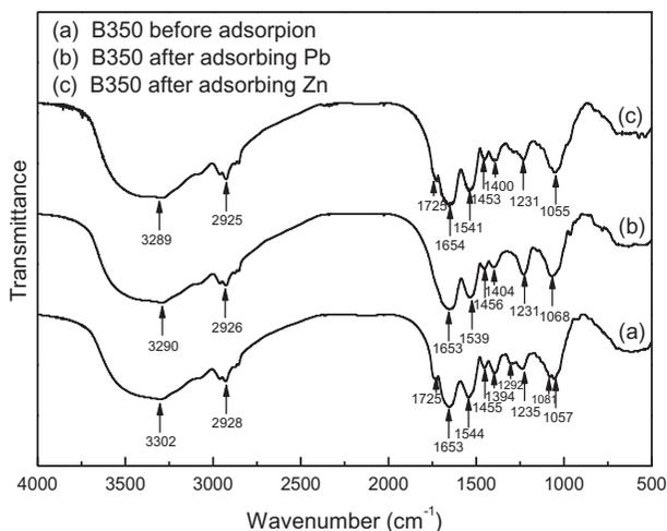
Fig. 5. FTIR spectra of B350 before and after adsorption.
