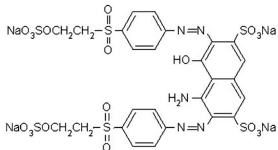
Fig. 1. Chemical structure Reactive Black 5.
