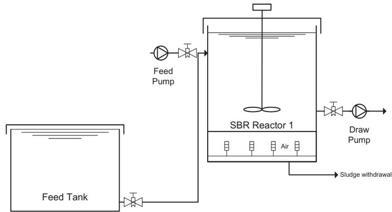
Fig. 2. Scheme of the SBR laboratory plant.
