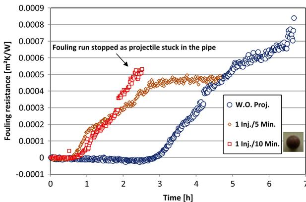
Fig. 5. Impact of P04 on fouling resistance for different injection intervals. (Bulk temperature 40°C, velocity 1.3 m/s, surface temperature 71°C and concentration 4.6 g/l).
