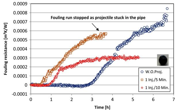
Fig. 6. Impact of P11 on fouling resistance at different injection frequencies. (Bulk temperature 40°C, velocity 1.3 m/s, surface temperature 71°C and concentration 4.6 g/l).
