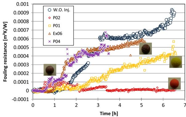
Fig. 4. Comparison of various projectiles on cleaning for the same injection intervals of 5 min. (Bulk temperature 40°C, velocity 0.8 m/s, surface temperature 80°C, concentration 3.8 g/l).
