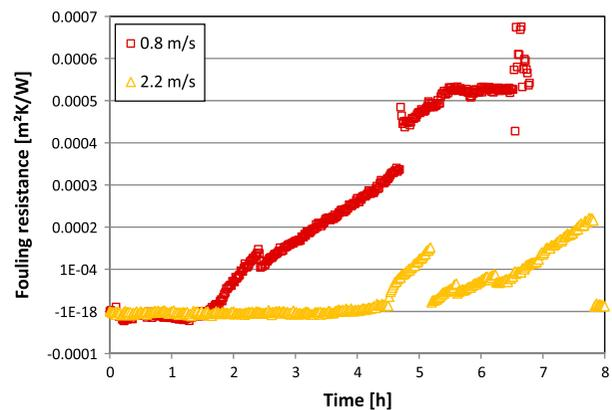
Fig. 3. Fouling resistance vs. time for different velocities without injecting projectiles. (Bulk and surface temperature of 40 and 80°C and concentration of 3.8 g/l).
