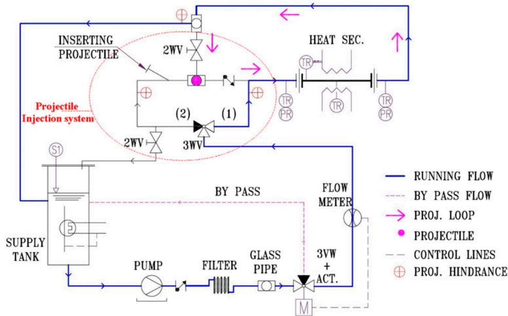
Fig. 1. Flow diagram of the fouling test facility.
