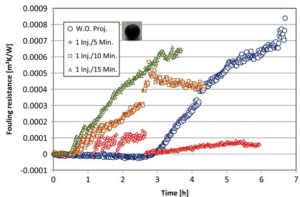
Fig. 7. Effect of P12 on cleaning for different injection frequencies. (Bulk temperature 40°C, velocity 1.3 m/s, surface temperature 71°C and concentration 4.6 g/l).
