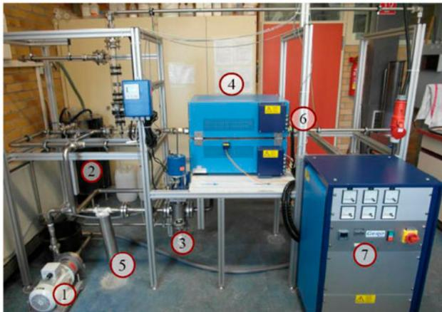
Fig. 2. A photo of the experimental setup, (1) 3 hp centrifugal pump, (2) 601 supply tank, (3) a 3 WV that is fully actuated by a motor and a flow controller, (4) a 10 kW electrical furnace, (5) 70  $\mu\text{m}$  filter, (6) piping and (7) control panel of the furnace.
