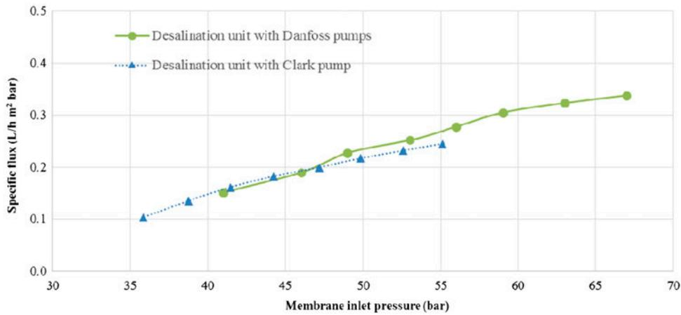
Fig. 4. Specific flux as a function of the membrane inlet pressure.
