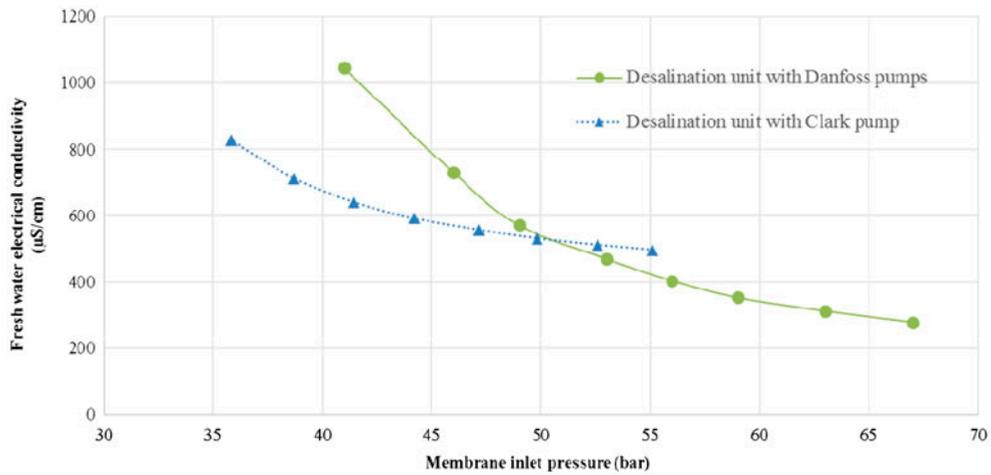
Fig. 5. Fresh water quality as a function of the membrane inlet pressure.
