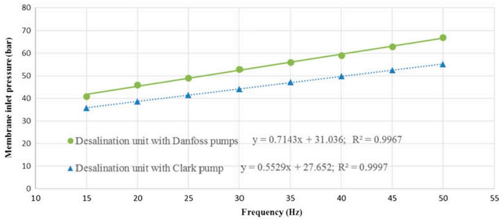
Fig. 3. Membrane inlet pressure as a function of the frequency of the motor.
