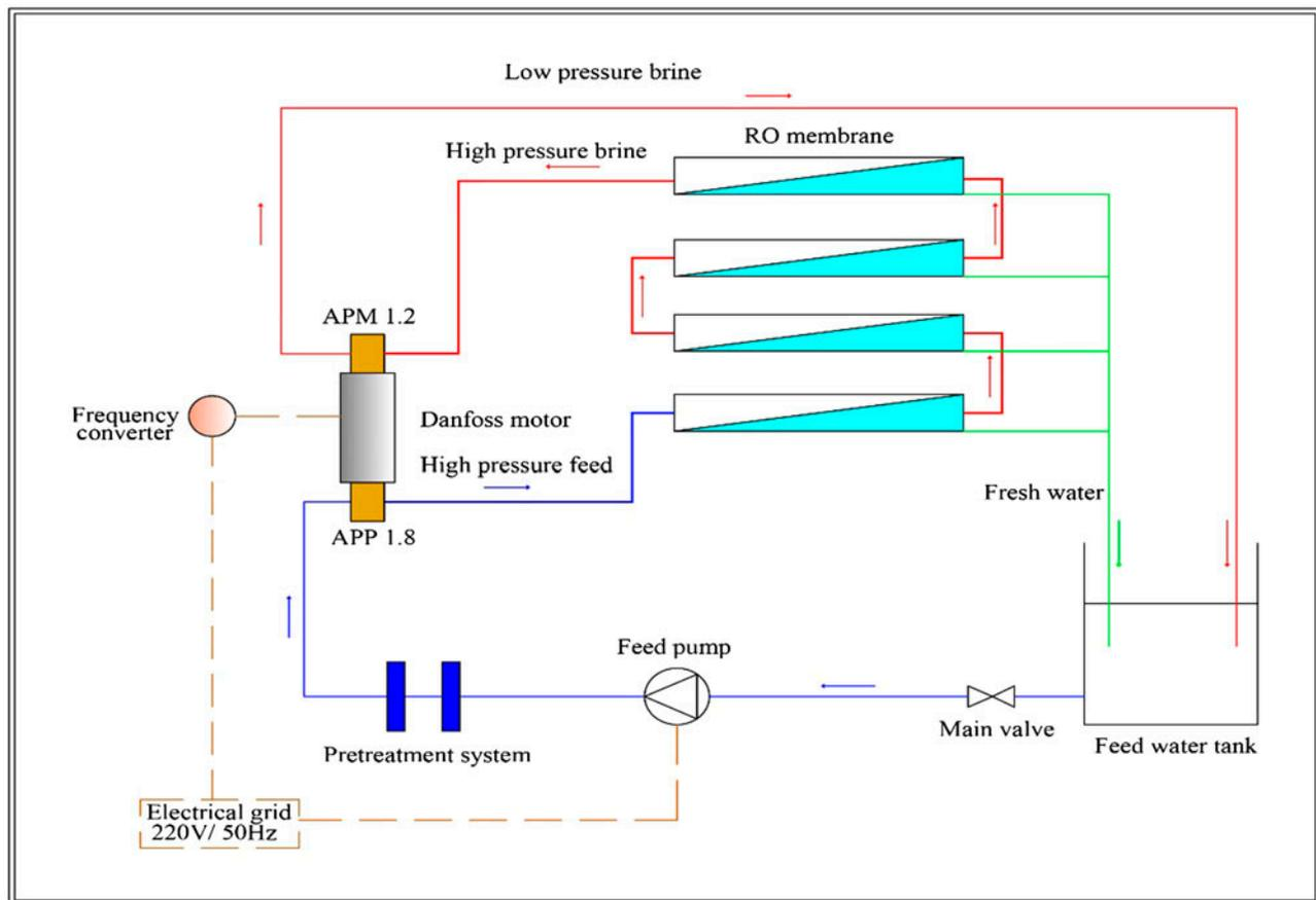
Fig. 2. Schematic diagram of the second desalination unit.
