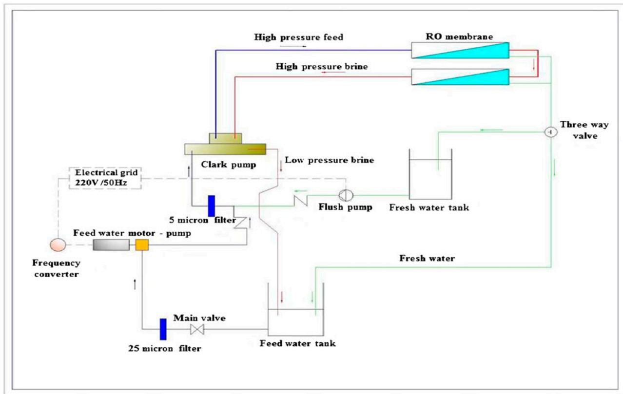
Fig. 1. Schematic diagram of the first desalination system.
