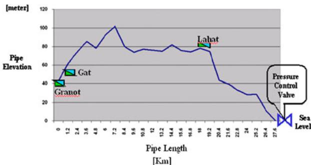
Fig. 6. A topographic section of the brine disposal pipeline and the Gat, Granot, and Lahat desalination plants. Source: [3].
