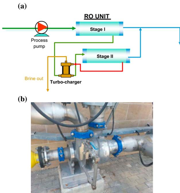
Fig. 8. (a) A schematic illustration of a two stage BWRO system with an interstage TC. (b) A photo of one of the TCs in Lahat 1 and 2 plants.
