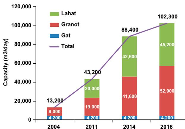
Fig. 3. Capacities of the Gat, Granot, and Lahat BWRO desalination plants throughout the years of 2004–2016.
