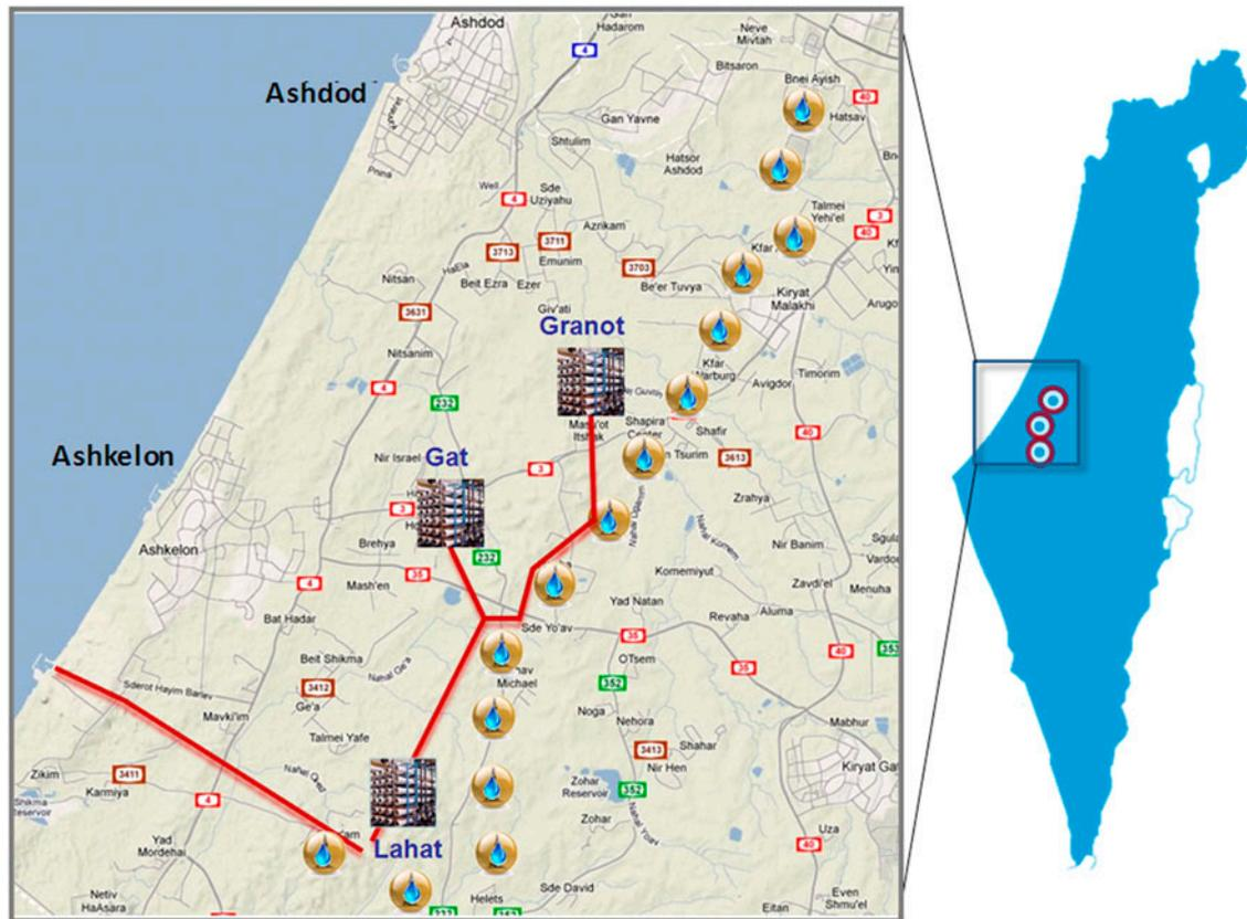
Fig. 5. The southern coastal aquifer rehabilitation project—a schematic map of the location of the new wells (yellow circles), the Gat, Granot, and Lahat desalination plants, and the brine disposal pipeline (red line). Source: [2].
