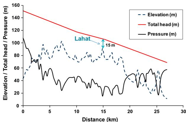
Fig. 7. The future total head line (red), changing elevations (dashed blue line), and designed pressures (black line) along the Granot to Ashkelon pipeline.
