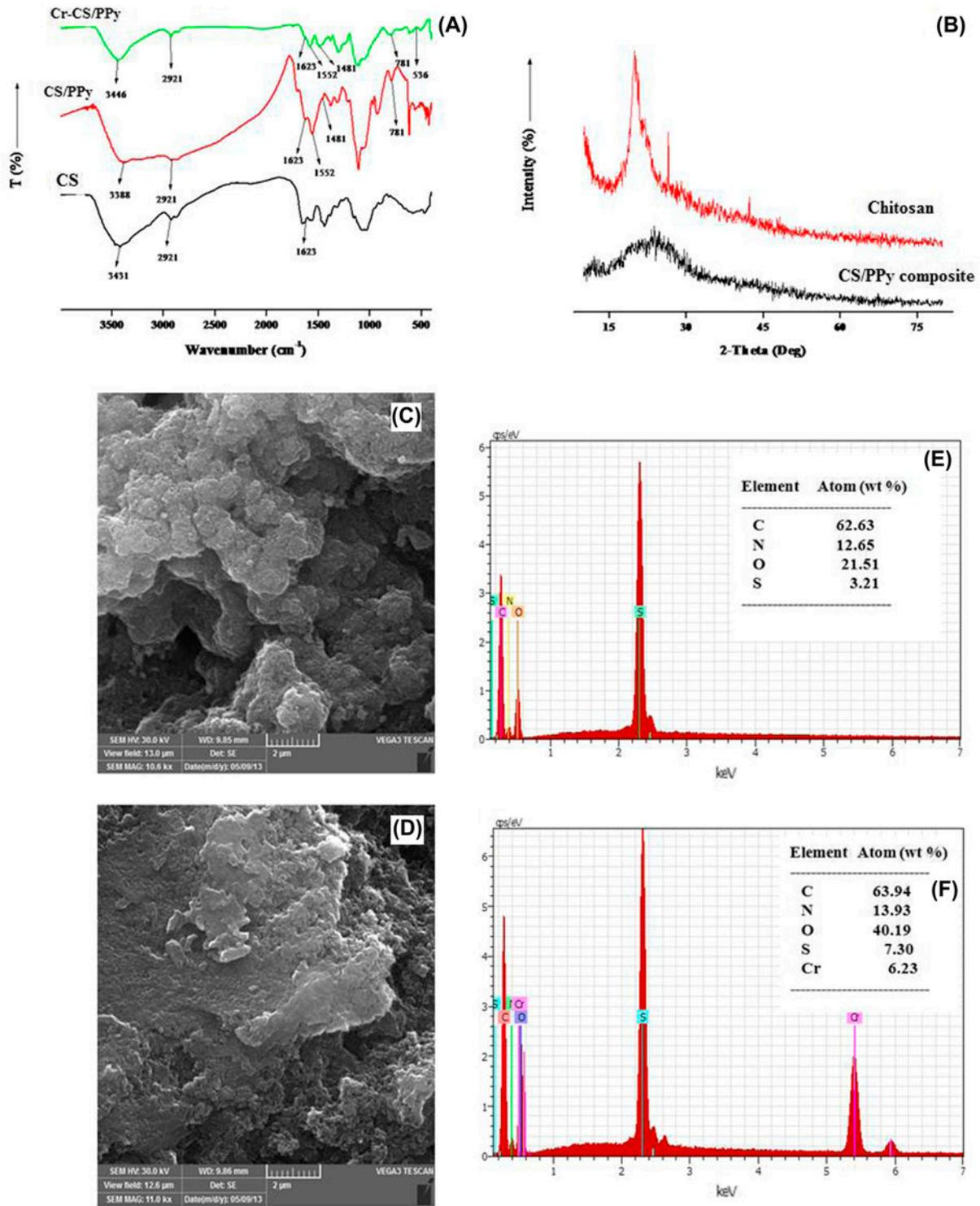
Fig. 1. (A) FTIR spectra of CS, CS/PPy, and Cr-CS/PPy composite, (B) XRD pattern of CS and CS/PPy composite, (C and D) SEM micrographs of CS/PPy and Cr-CS/PPy composite, and (E and F) EDX spectra of CS/PPy and Cr-CS/PPy composite.
