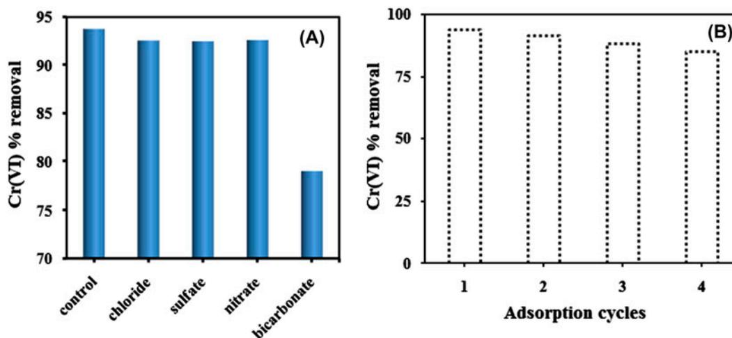
Fig. 4. (A) Effect of co-anions on the removal of Cr(VI) ions by CS/PPy composite and (B) Desorption–regeneration cycles.
