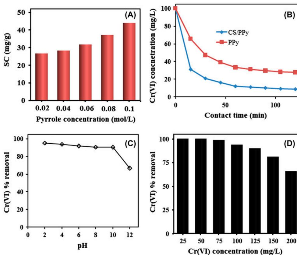
Fig. 2. Optimization of various parameters for the removal of Cr(VI) ions by CS/PPy composite (A) Effect of pyrrole concentration, (B) Effect of contact time, (C) Influence of pH, and (D) Effect of initial concentration.
