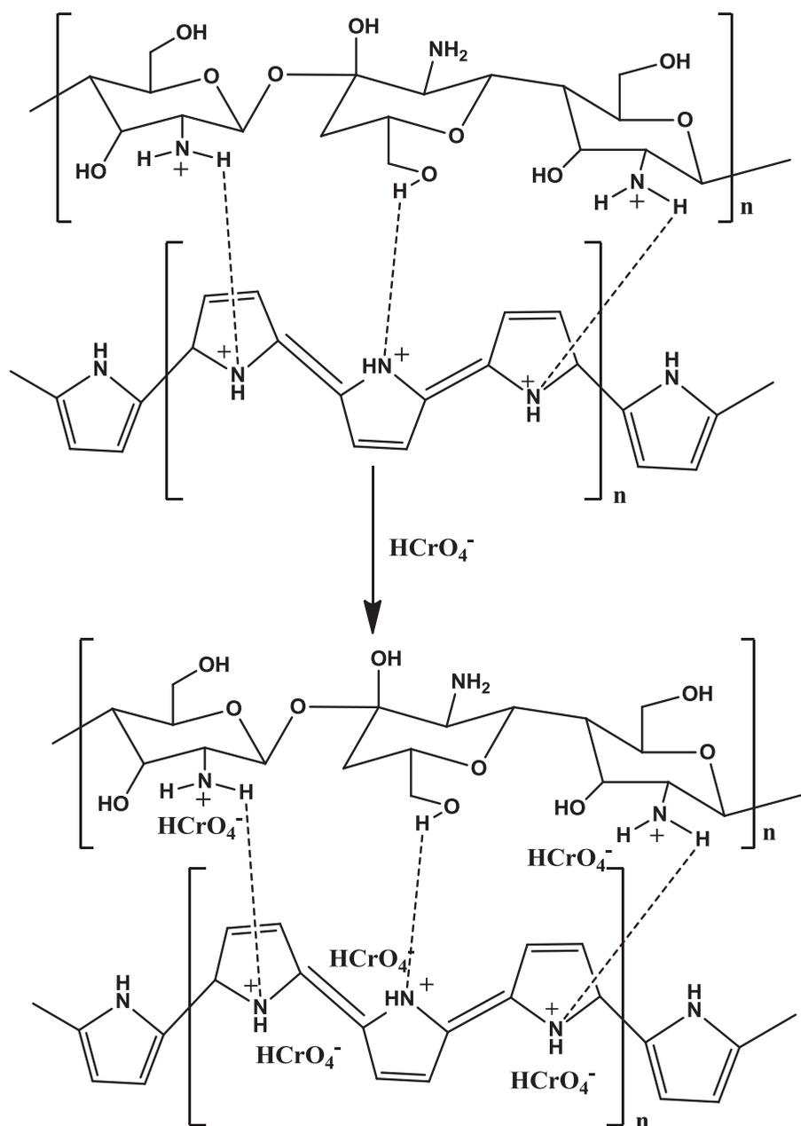
Scheme 1. Mechanism of Cr(VI) ion removal by CS/PPy composite.
