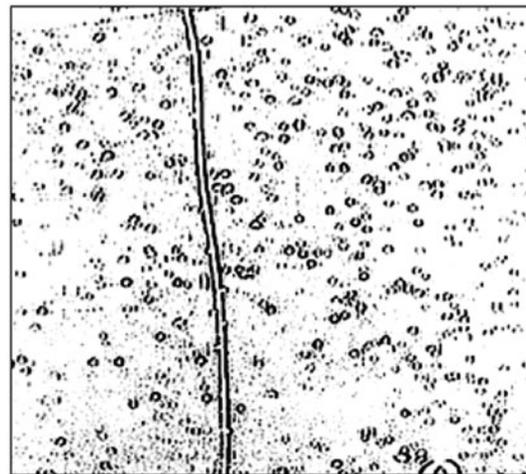
Fig. 3. Image treated for the determination of bubble size.
