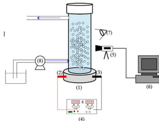
Fig. 2. Electroflotation column and equipment for the determination of bubble characteristic in continuous mode (co-current configuration).
