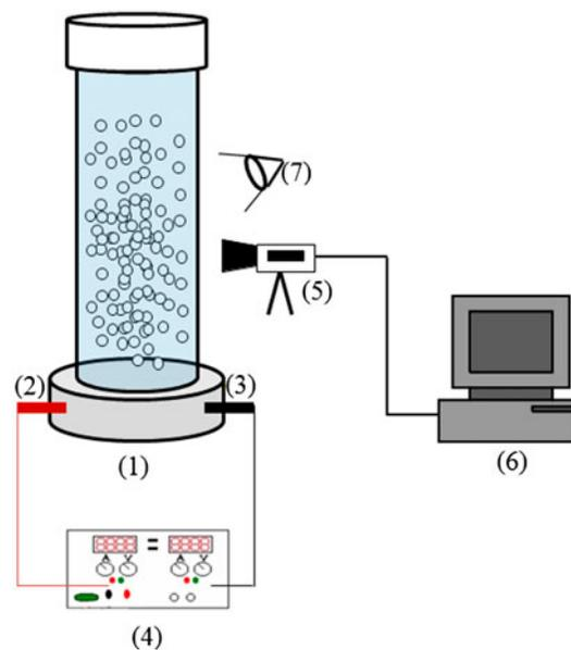
Fig. 1. Electroflotation column and equipment for the determination of bubble characteristic in batch mode.
