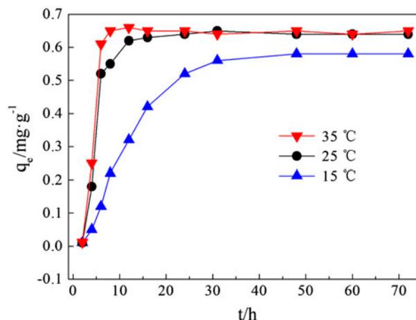
Fig. 2. The kinetics of phosphorus adsorption of EPRC at different temperatures (Conditions: EPRC particle size 0.5 cm; initial P concentration 5 mg/L; mixing rate 100 rpm).
