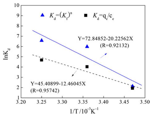
Fig. 4. The influence of temperature on the equilibrium adsorption coefficients.
