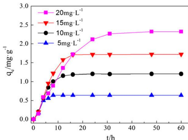
Fig. 1. The kinetics of phosphorus adsorption of EPRC at different initial phosphorus concentrations (Conditions: EPRC particle size 0.5 cm; concentration 8 g/L; mixing rate 100 rpm, 25 °C).
