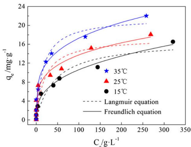
Fig. 3. The adsorption isotherms of EPRC (Conditions: EPRC particle size 0.5 cm; concentration 4 g/L; mixing rate 100 rpm).
