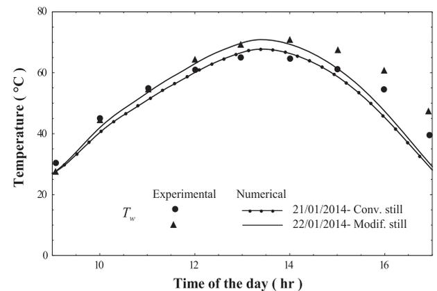
Fig. 6. Experimental and numerical temperature variations of brackish water for the two solar stills.
