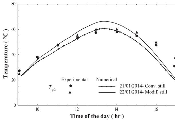
Fig. 7. Experimental and numerical temperature variations of glass cover for the two solar stills.
