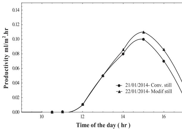
Fig. 8. Variation of fresh water productivity for the two solar stills.
