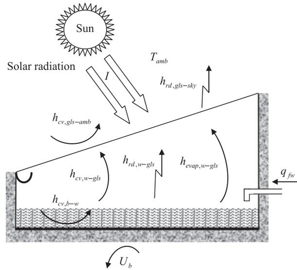
Fig. 3. Schematic diagram of heat transfer mechanisms in the solar still.
