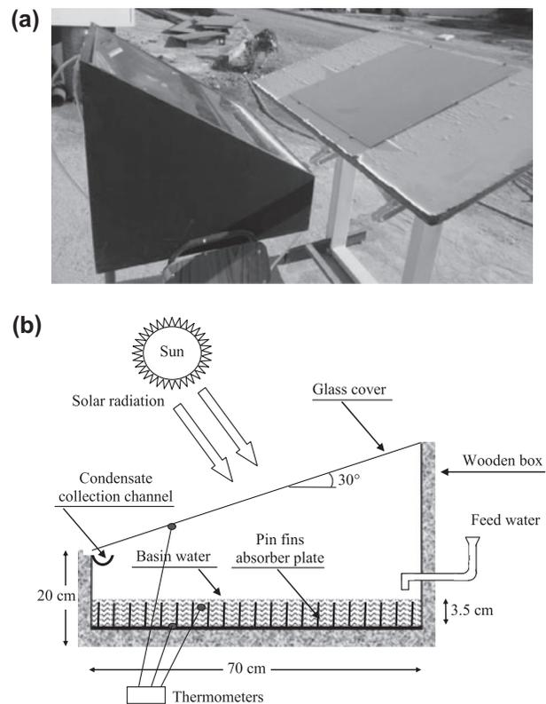
Fig. 1. (a) Solar still with moving mirror. (b) Cross-section of a solar still experimental setup.
