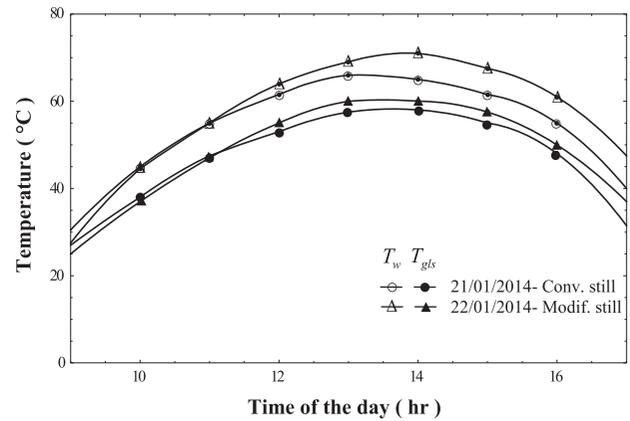
Fig. 5. Experimental temperature variations of water and glass for the modified and conventional still.
