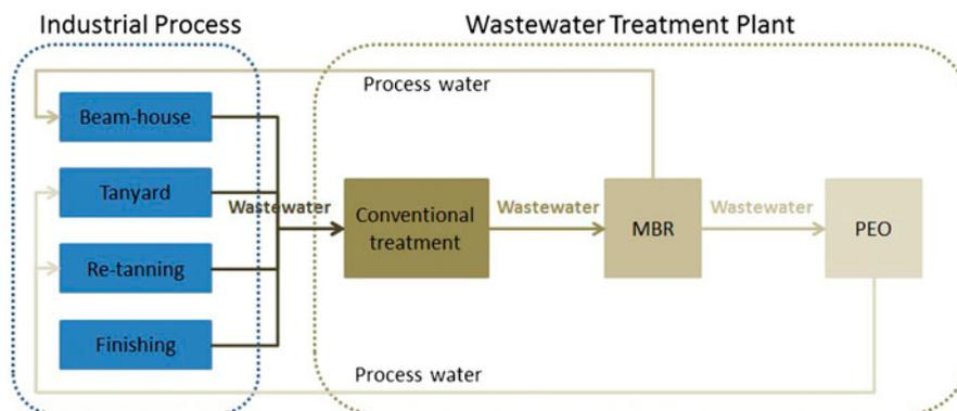
Fig. 9. Proposal of wastewater treatment and water reuse in a tannery.
