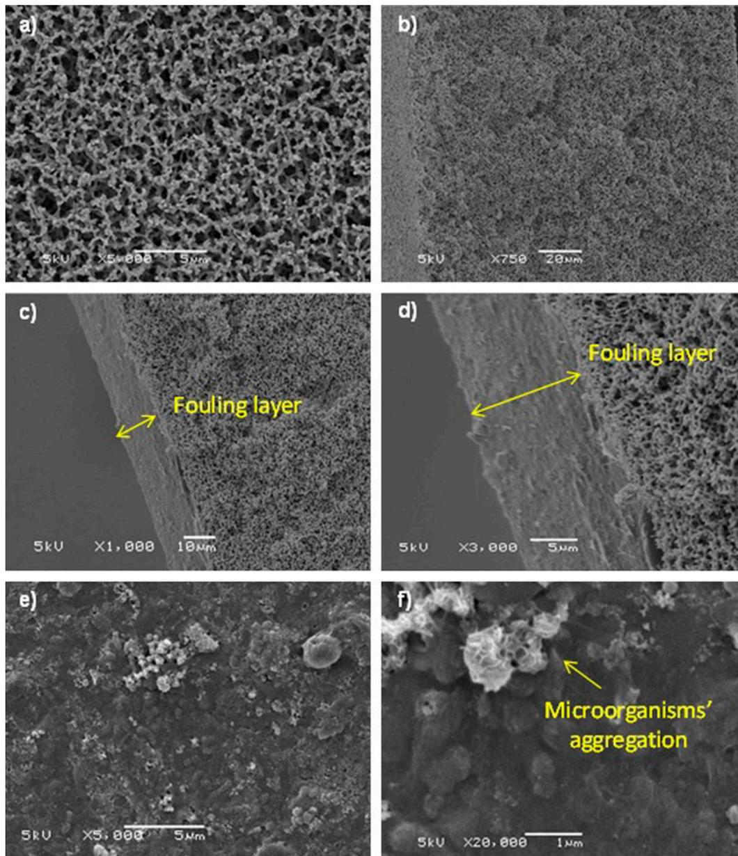
Fig. 5. SEM images of the membrane: ((a) and (b)) surface and cross-section of the new membrane; ((c) and (d)) cross-section of fouled membrane; ((e) and (f)) surface of fouled membrane.
