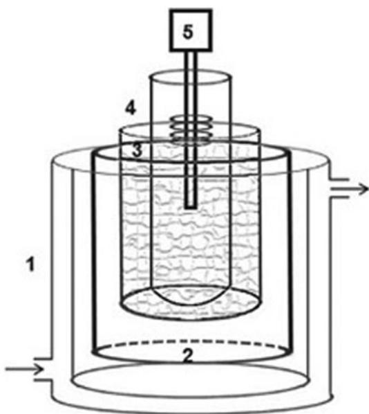
Fig. 3. Schematic representation of photoreactor: (1) glass reservoir; (2) titanium oxide cathode; (3) titanium and ruthenium oxides anode; (4) quartz tube; and (5) mercury vapour lamp.
