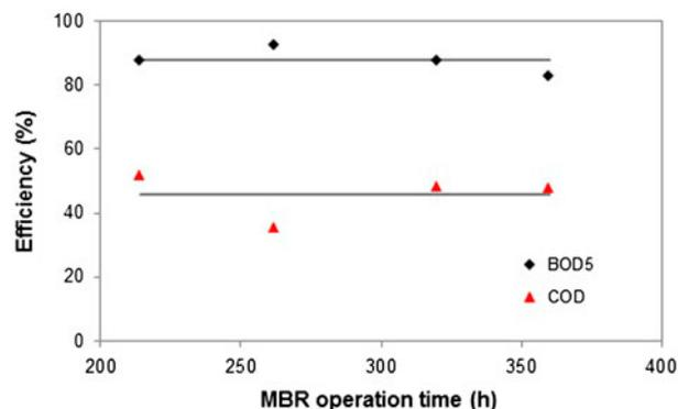
Fig. 8. MBR efficiency treating the tannery wastewater.
