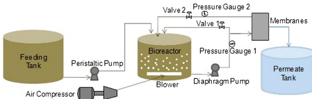
Fig. 2. MBR experimental set-up.
