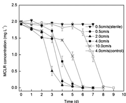
Fig. 4. MC-LR biodegradation curves by EFB sediment at different flow rates, 0.5 cm/s (sterile group) (dark inverted triangle), 0.5 cm/s (dark closed circles), 2.0 cm/s (dark triangle), 4.0 cm/s (dark square), 10.0 cm/s (X-type), and 4.0 cm/s (control group) (white square), under anoxic condition at 25°C. Error bars represent the range of duplicate samples.
