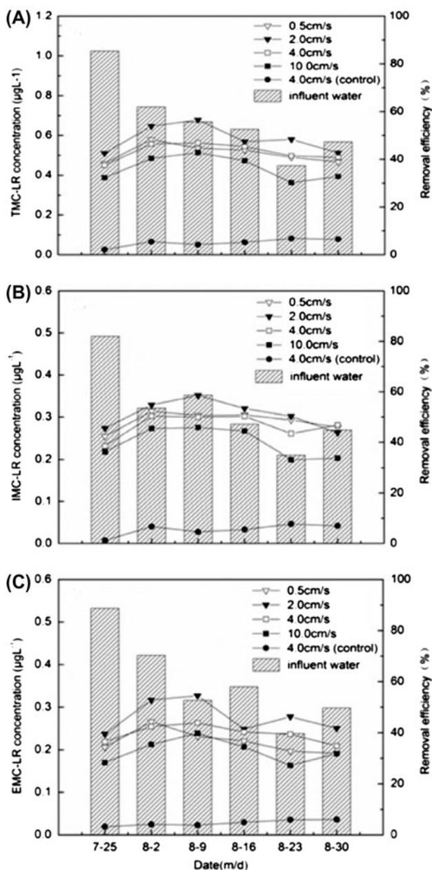
Fig. 2. Removal efficiency and influent concentration of (A) total- (B) intracellular- and (C) extracellular-MC-LR at different flow rates, 0.5 cm/s (white inverted triangle), 2.0 cm/s (dark inverted triangle), 4.0 cm/s (white square), 10.0 cm/s (dark square), and 4.0 cm/s (control group) (dark closed circles).
