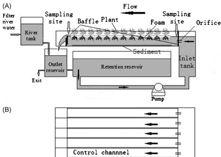
Fig. 1. Laboratory simulation of EFB system. (A) The side view of the EFB system. (B) The plan view of the EFB system.
