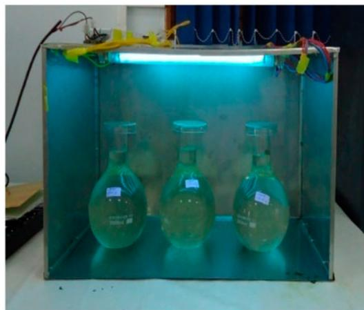
Fig. 1. 2 L-flasks under UV radiation.
