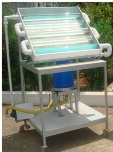
Fig. 3. 30 L-tubular photoreactor under solar radiation.
