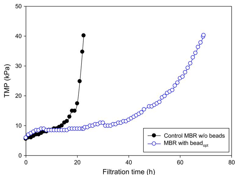
Fig. 5. Effect of fully optimized bead condition (bead<sub>opt</sub>) on the MBR performance.
