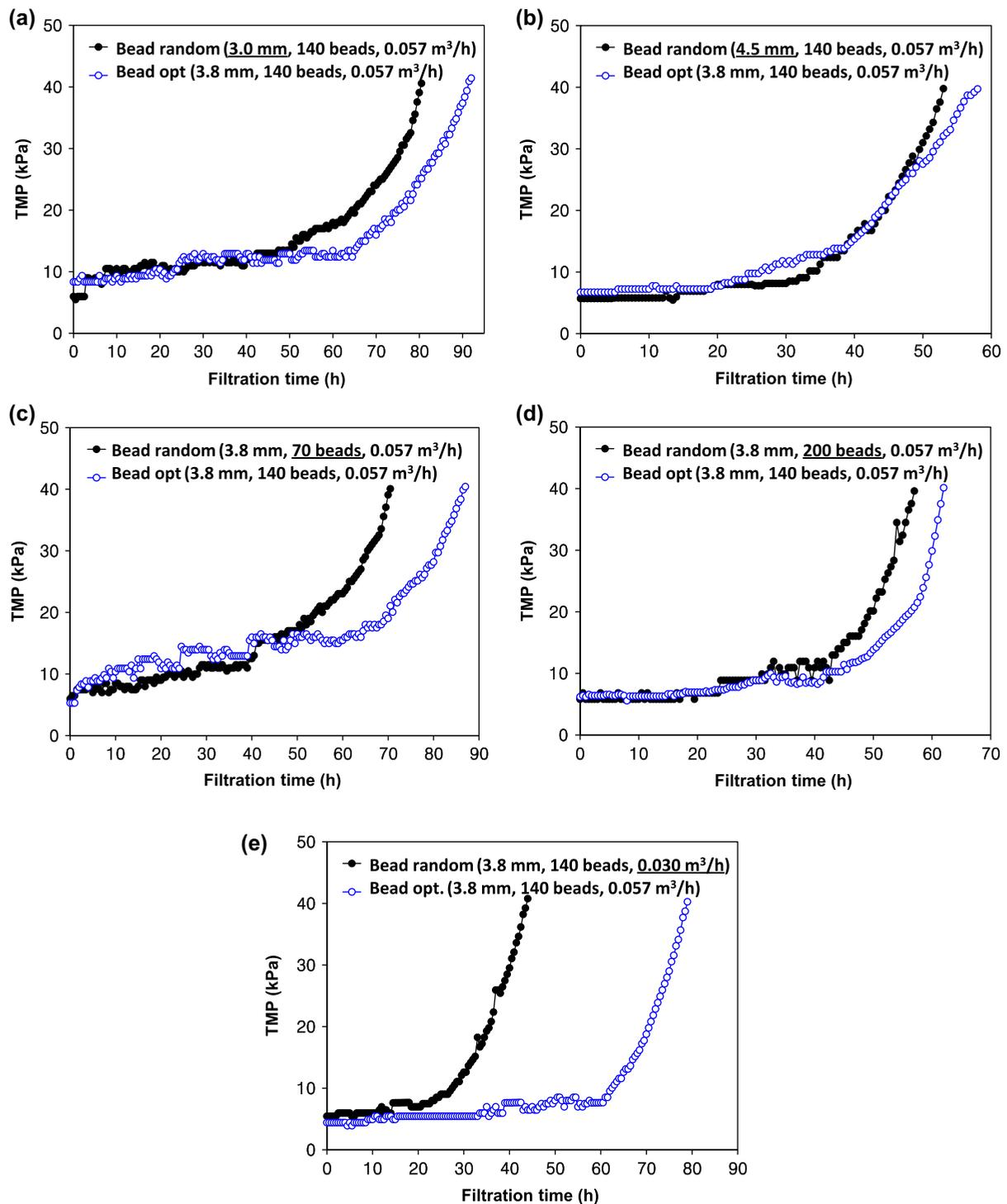
Fig. 6. Effect of partial variance of single parameter on the MBR performance. (a) Low diameter level (3.0 mm), (b) high diameter level (4.5 mm), (c) low number level (70 beads), (d) high number level (200 beads), and (e) low aeration level (0.030 m<sup>3</sup>/h).
