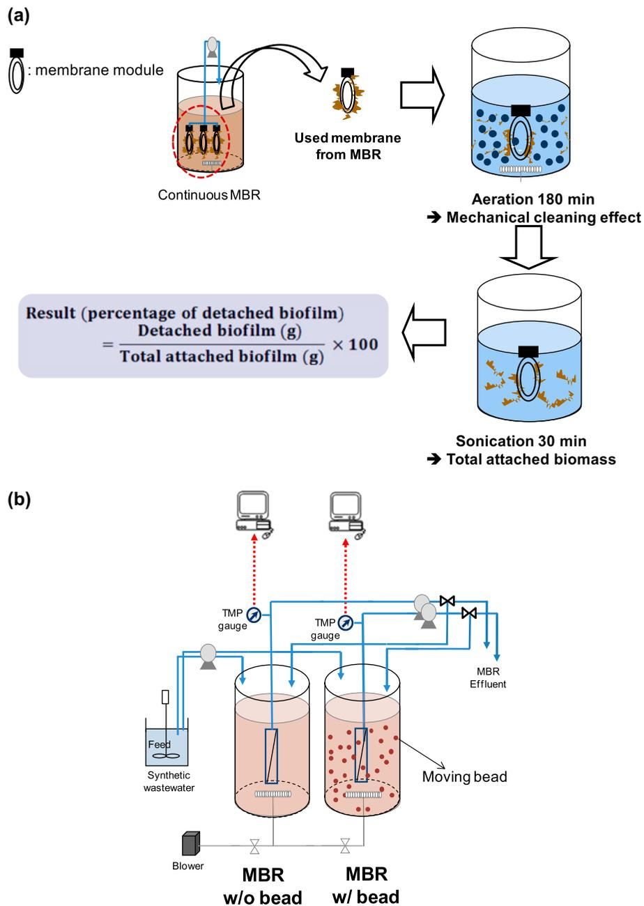
Fig. 1. Schematic diagram of (a) batch reactor for bio-cake detachment and (b) parallel operation of lab-scale MBRs.
