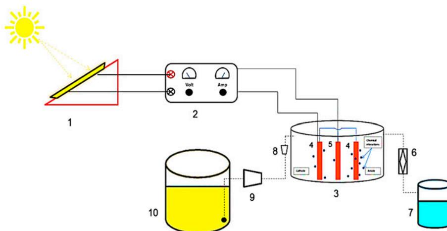
Fig. 1. Diagram of the experimental setup. 1. PV Solar module, 2. Regulator, 3. Electrocoagulation reactor, 4. Electrode (a), 5. Electrode (b), 6. Filter, 7. Treated solution, 8. Flow meter, 9. Peristaltic pump, and 10. Wastewater deposit.
