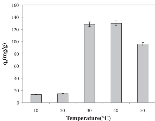
Fig. 3. Effect of temperature on the adsorption of methylene blue ( $K_2HPO_4$  concentration: 2 M, impregnation time: 6 h, and impregnation ratio: 0.05).
