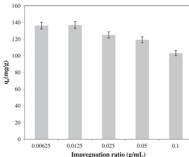
Fig. 4. Effect of different impregnation ratio on the adsorption of methylene blue ( $K_2HPO_4$  concentration: 2 M, impregnation time: 6 h, and temperature: 30°C).
