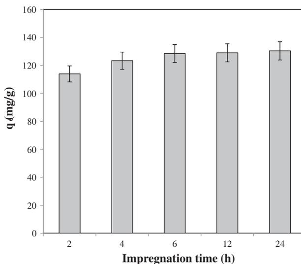
Fig. 2. Effect of impregnation time on the adsorption of methylene blue ( $K_2HPO_4$  concentration: 2 M, impregnation ratio: 0.05, and temperature: 30 °C).
