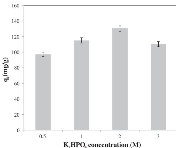
Fig. 1. Effect of  $K_2HPO_4$  concentration on the adsorption of methylene blue (impregnation time: 24 h, impregnation ratio: 0.05, and temperature: 30 °C).
