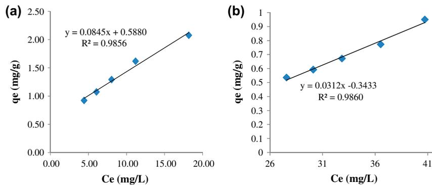
Fig. 5. Langmuir isotherm model plot of nitrate on GAC (a) and on NZM (b), 300 rpm, 20°C, and 30 min contact time.
