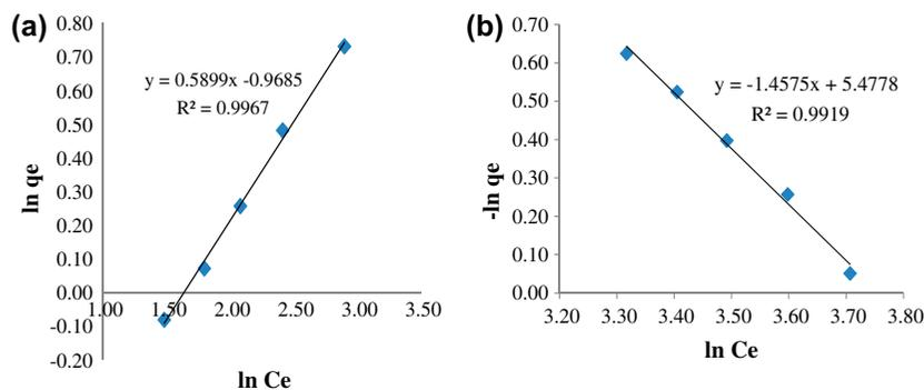
Fig. 6. Langmuir isotherm model plot of  $\text{NO}_3^-$  on GAC (a) and on NZM (b), 300 rpm, 20°C, and 30 min contact time.
