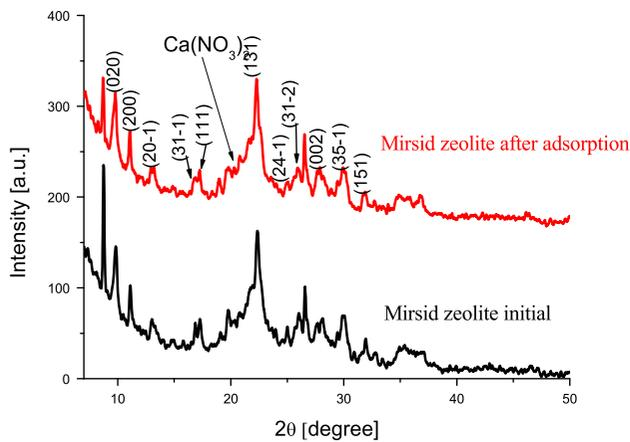
Fig. 8. X-ray powder diffraction patterns for initial NZM and after adsorption.
