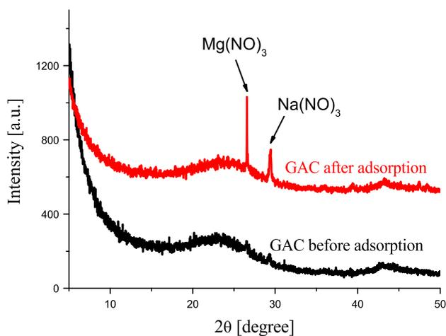
Fig. 9. X-ray powder diffraction patterns for initial GAC and after adsorption.
