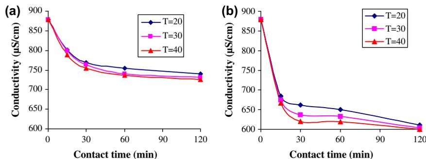
Fig. 2. The conductivity of the groundwater vs. the adsorption time at different adsorption temperatures (20, 30, and 40°C), 300 rpm, for NZM (a) and GAC adsorber (b).
