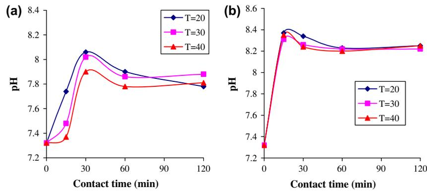
Fig. 1. The pH of treated groundwater as a function of adsorption time at different adsorption temperatures (20, 30, and 40°C), 300 rpm, for NZM (a) and GAC adsorber (b).
