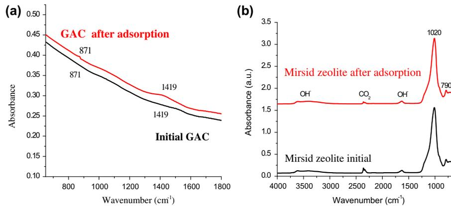
Fig. 7. FTIR-spectra of GAC (a) and NZM (b) before and after the groundwater adsorption treatment.
