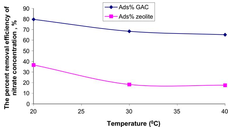
Fig. 4. The value for percent removal of  $\text{NO}_3^-$  after 30 min contact time.
