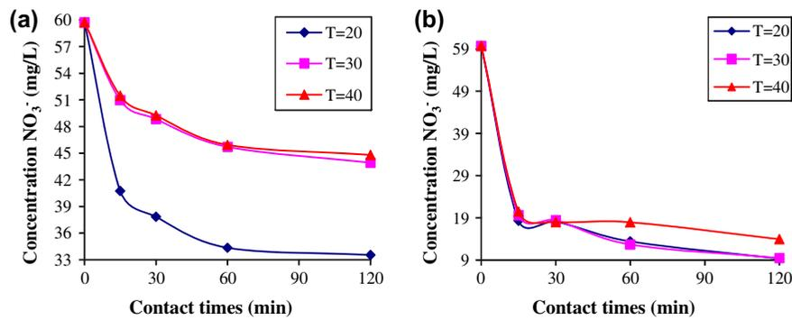
Fig. 3. The concentration of nitrate from treated water as a function of adsorption time at different temperatures (20, 30, and 40°C), 300 rpm, for NZM (a) GAC (b) adsorbent.
