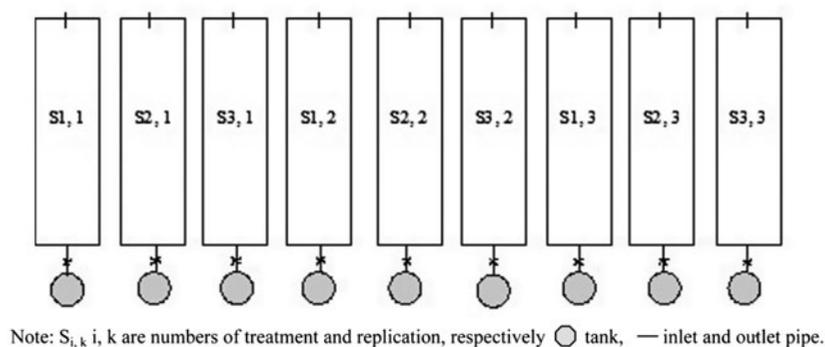
Fig. 1. Layout of CW systems.
