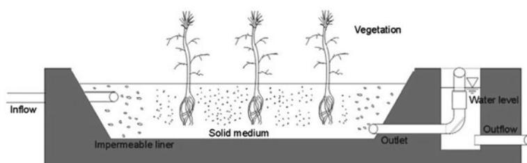
Fig. 2. Longitudinal cross section of a horizontal flow CW.
