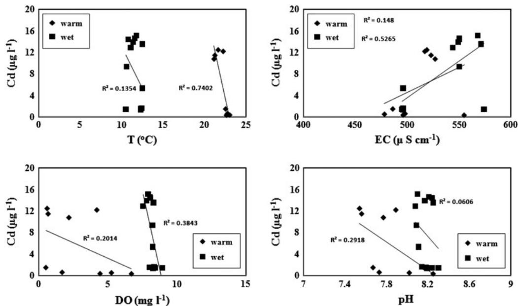
Fig. 7. Linear relationship between dissolved Cd and physicochemical parameters in Shahid Rajaei dam's reservoir in hypolimnion.
