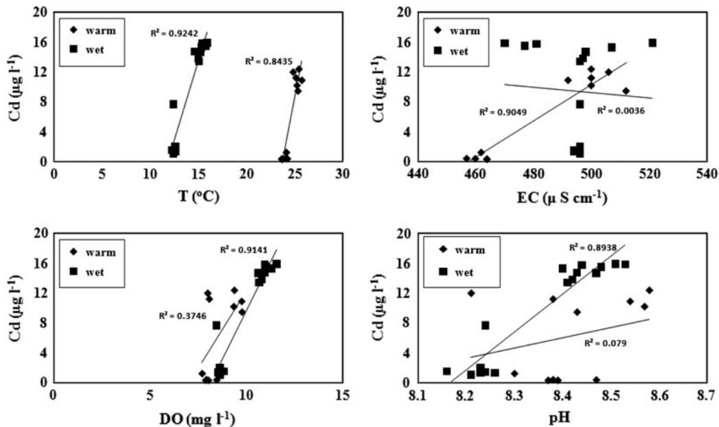
Fig. 5. Linear relationship between dissolved Cd and physicochemical parameters in Shahid Rajaei dam's reservoir in epilimnion.
