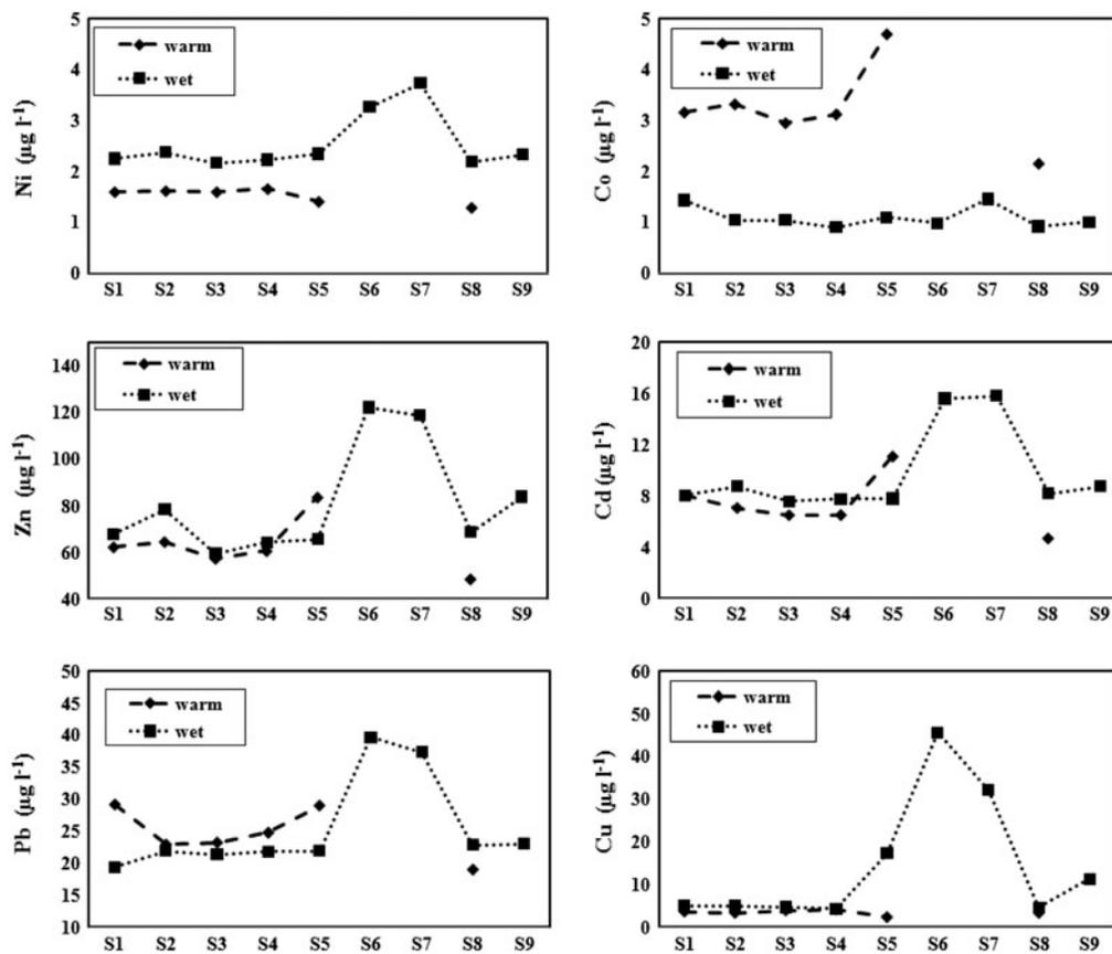
Fig. 4. Spatial pattern of the dissolved heavy metals concentrations (mean values) in the Shahid Rajaei dam's reservoir, Iran.
