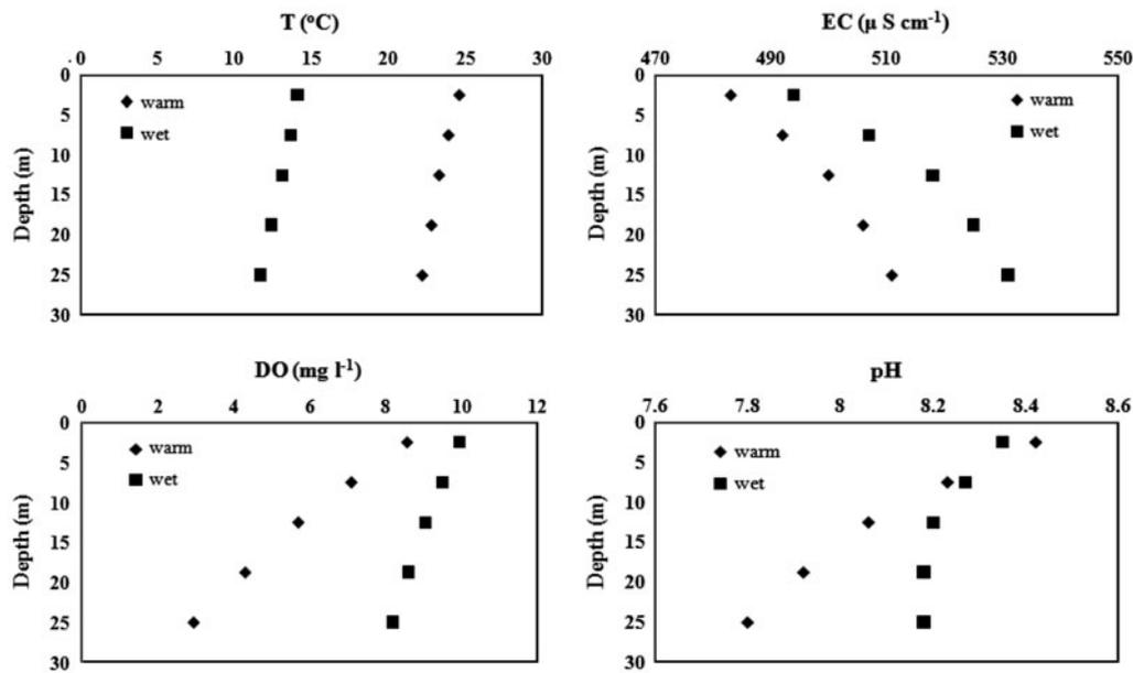
Fig. 2. Variation of physicochemical parameters with depth of Shahid Rajaei dam's reservoir.
