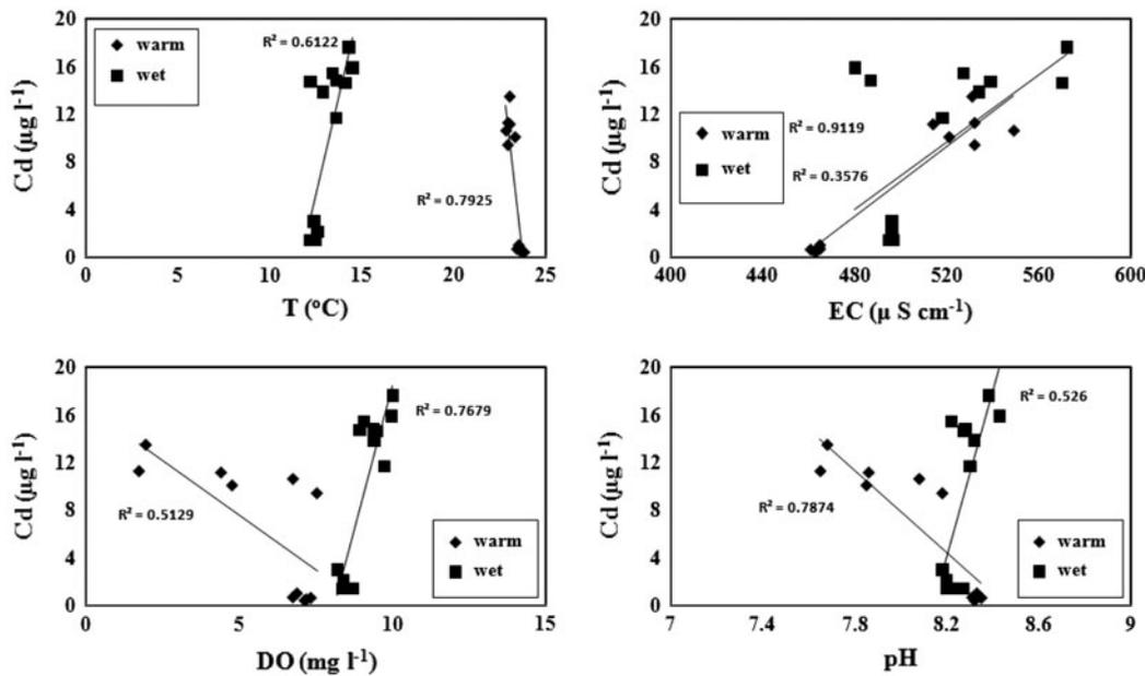
Fig. 6. Linear relationship between dissolved Cd and physicochemical parameters in Shahid Rajaei dam's reservoir in metalimnion.
