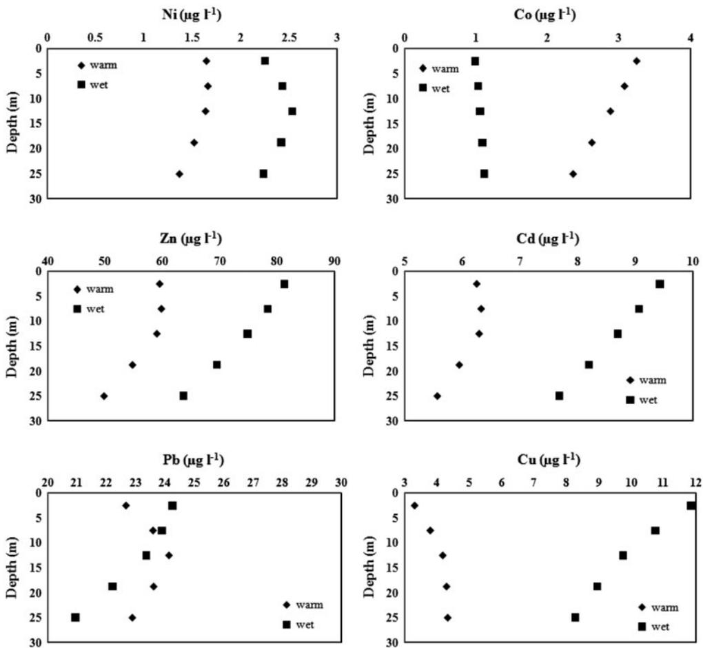
Fig. 3. Variation of dissolved heavy metals concentrations with depth of Shahid Rajaei dam's reservoir.
