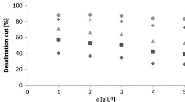
Fig. 8. Dependence of desalination cut on inlet NaCl concentration at linear flow velocity of  $5.9 \text{ cm s}^{-1}$  and voltages of  $\blacklozenge$  12.5 V,  $\blacksquare$  18.75 V,  $\blacktriangle$  25 V,  $+$  37.5 V, and  $\bullet$  50 V.
