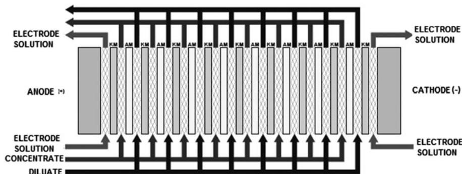
Fig. 1. Typical ED stack structure.
