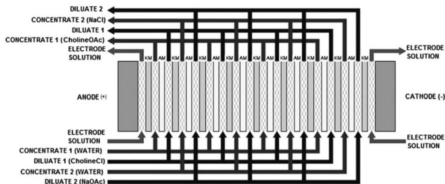
Fig. 4. Ionic liquid production by means of metathesis (four-circuit ED stack).
