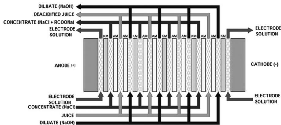
Fig. 3. Three-circuit ED stack for juice deacidification.
