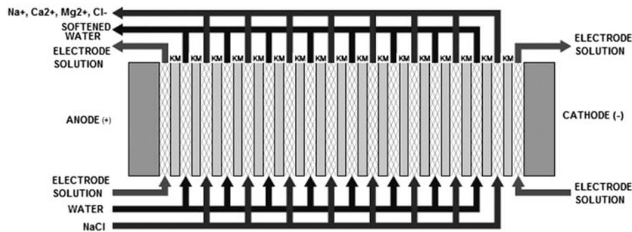
Fig. 2. ED stack composed of CEMs for water softening.
