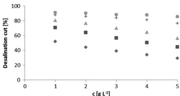
Fig. 7. Dependence of desalination cut on inlet NaCl concentration at linear flow velocity of  $4.4 \text{ cm s}^{-1}$  and voltages of  $\blacklozenge$  12.5 V,  $\blacksquare$  18.75 V,  $\blacktriangle$  25 V,  $+$  37.5 V, and  $\bullet$  50 V.
