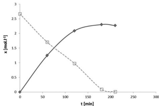
Fig. 6. Concentration profiles of lactic acid (full line) and sodium ions (dashed line) in product stream in time.
