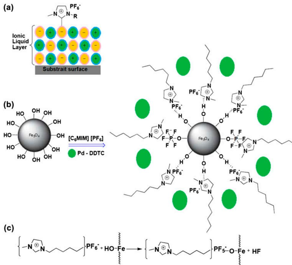
Fig. 4. The synthetic approach to prepare  $\text{Fe}_3\text{O}_4$  NPs-based supported IL.
