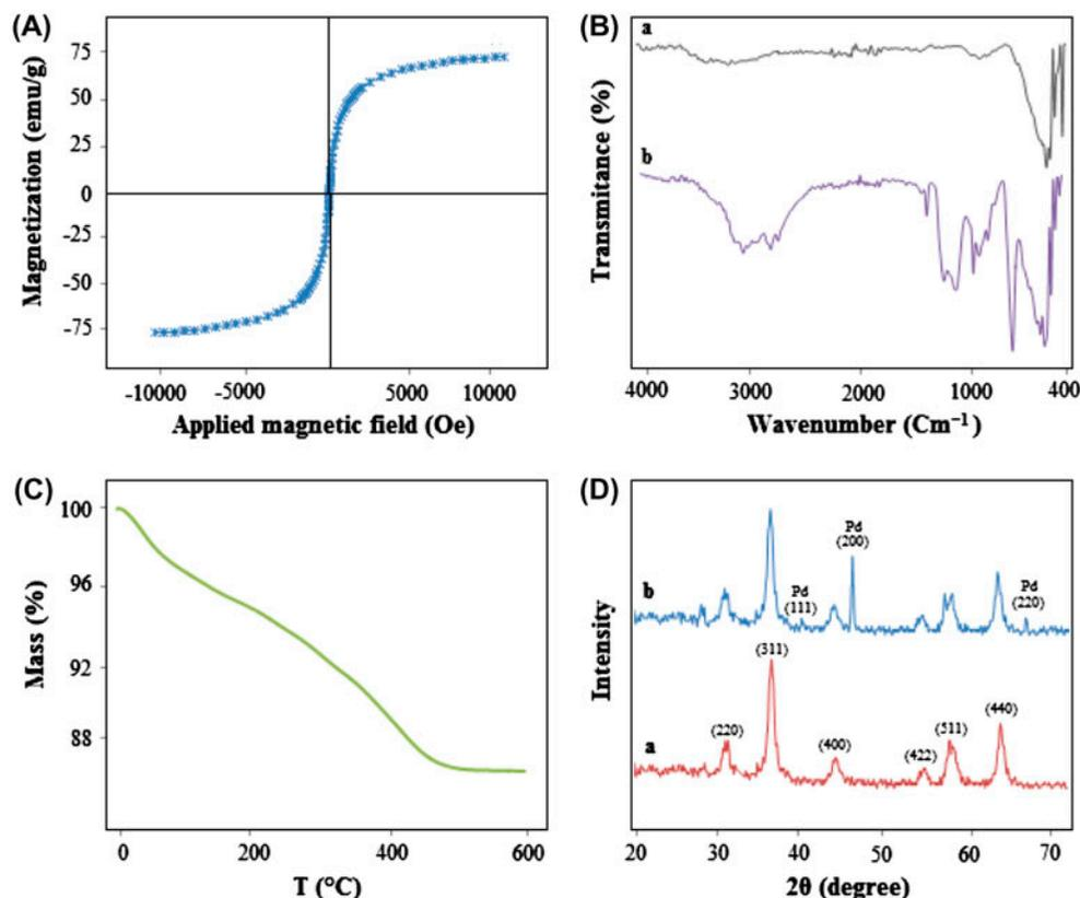
Fig. 3. (A) Magnetic hysteresis loops of  $\text{Fe}_3\text{O}_4$  NPs synthesized room temperature. (B) FTIR spectra of (a)  $\text{Fe}_3\text{O}_4$  NPs before modification and (b) IL-modified  $\text{Fe}_3\text{O}_4$  NPs. (C) The TGA curves for IL-modified  $\text{Fe}_3\text{O}_4$  NPs. (D) The XRD pattern for (a) synthesized  $\text{Fe}_3\text{O}_4$  NPs (b) IL-modified  $\text{Fe}_3\text{O}_4$  NPs equilibrated with palladium ions.
