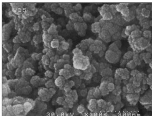
Fig. 1. SEM image of Fe<sub>3</sub>O<sub>4</sub> NPs prepared by ultrasonic chemical co-precipitation.
