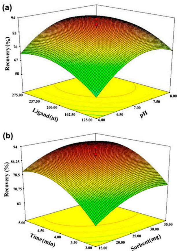
Fig. 5. (a) Three-dimensional response surface plot for the effect of pH and volume of ligand on the response (extraction recovery), in which the values of amount of adsorbent and time were fixed at 28 mg and 4 min, respectively. (b) Three-dimensional response surface plot for the effect of amount of adsorbent and time on the response (extraction recovery), in which pH and concentration of ligand were fixed at 7.6 and  $5.5 \times 10^{-6} \text{ mol L}^{-1}$  respectively.
