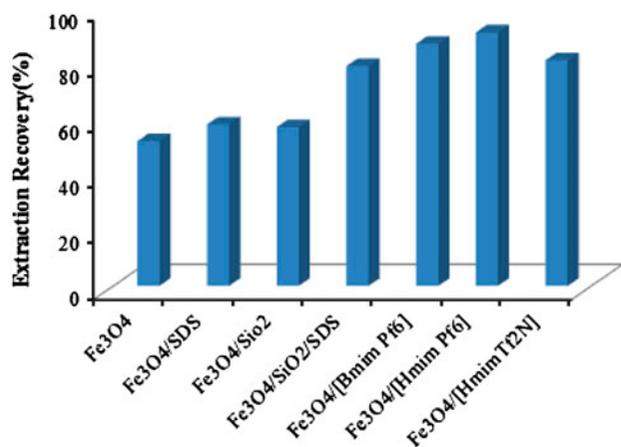
Fig. 2. Effect of different adsorbents on the extraction recovery of Pd(II). Condition: sample volume, 50 mL; Pd(II),  $100\text{ ng mL}^{-1}$ ; concentration of DDTC,  $5.5 \times 10^{-6}\text{ mol L}^{-1}$ ; pH 7.6; amount of adsorbent, 28 mg; and eluent volume (acetylacetone/ethanol (1:1)), 1 mL.
