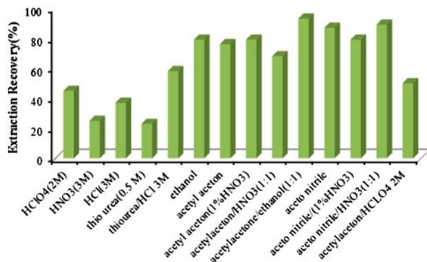
Fig. 6. Effect of different eluents on the extraction recovery of Pd(II). Condition: sample volume, 50 mL; Pd(II), 100  $\text{ng mL}^{-1}$ ; concentration of DDTC,  $5.5 \times 10^{-6} \text{ mol L}^{-1}$ ; pH 7.6; amount of adsorbent, 28 mg; and eluent volume, 1 mL.
