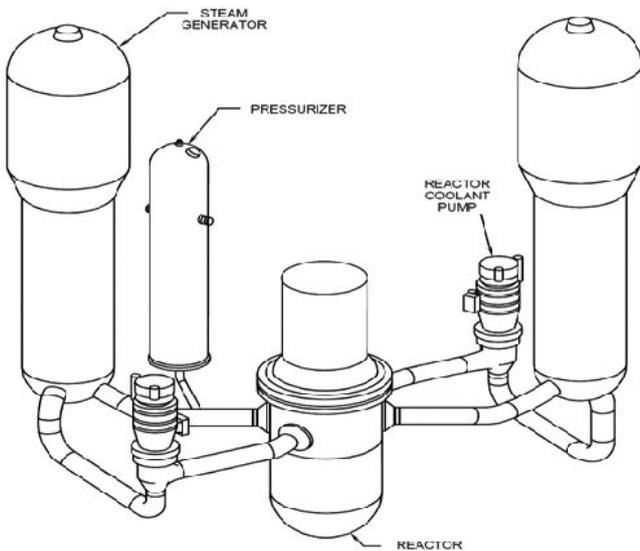
Fig. 7a. Sketch of the reactor combination with steam generator and pressurizer [9].
