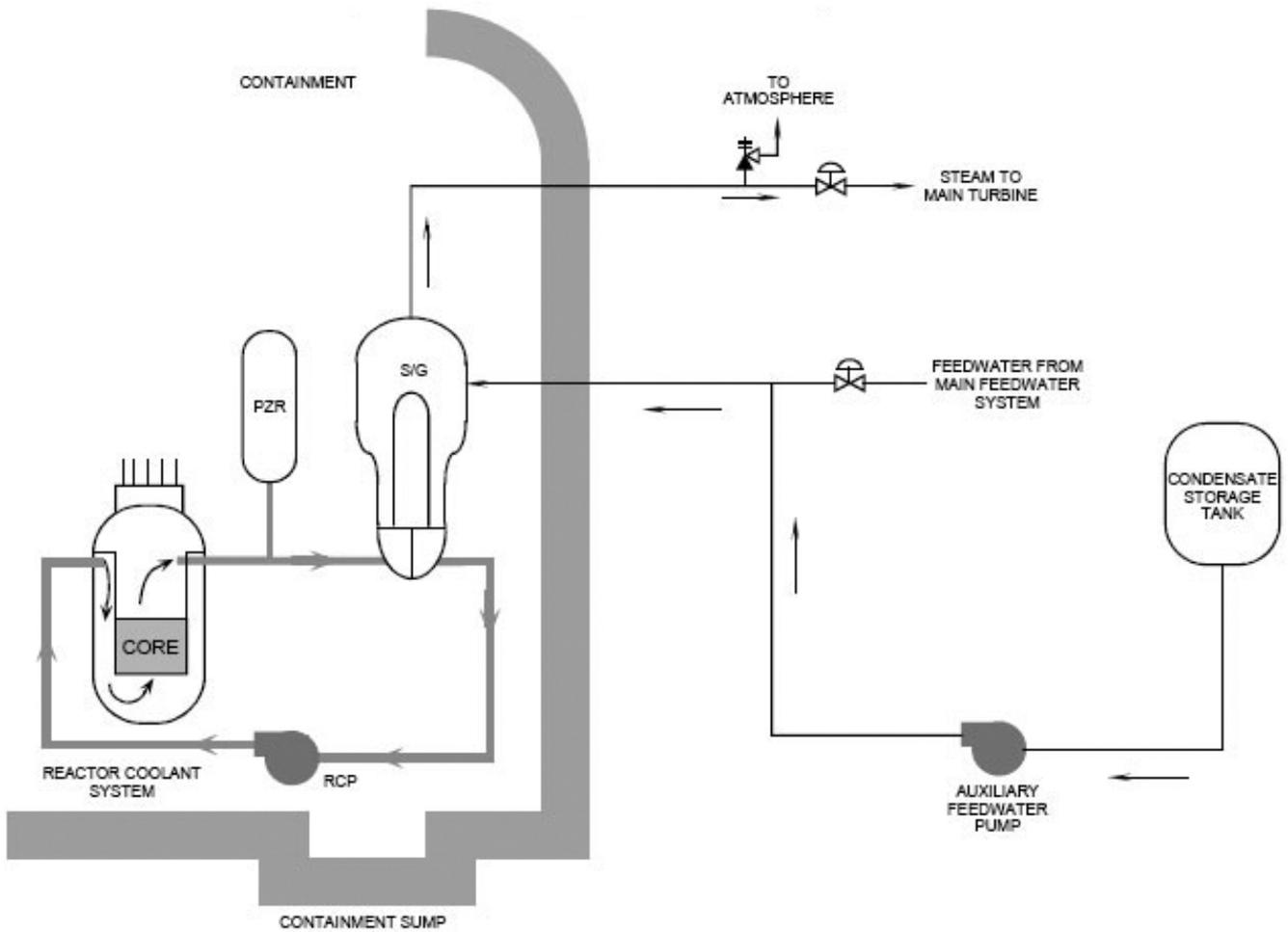
Fig. 8. Steam dump system used to decay heat removal.
