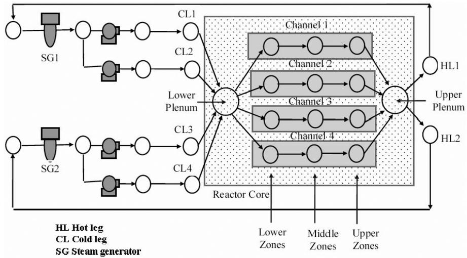
Fig. 7b. Primary loop (reactor coolant system) flow diagram [10].
