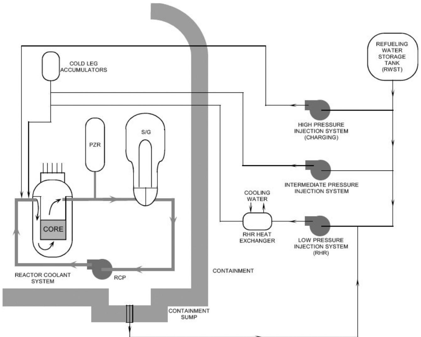
Fig. 9. Emergency cooling system by HP, IP, cold leg and LP.
