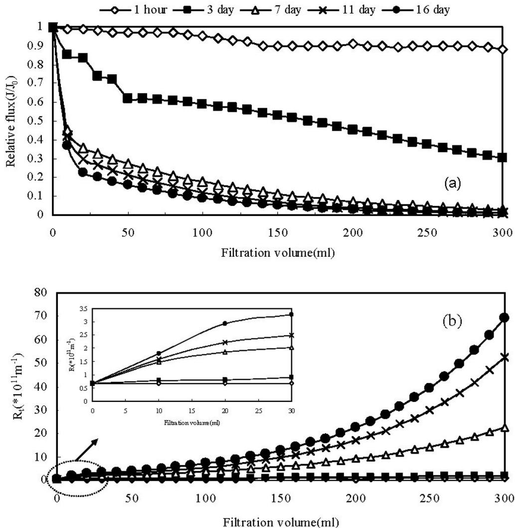
Fig. 4. Variations during the filtration of bulk solution. (a) Relative flux; (b) resistances ( $\Delta P$ : 1.0 bar; stirring rate: 180 rpm; temperature:  $20 \pm 2$ ).
