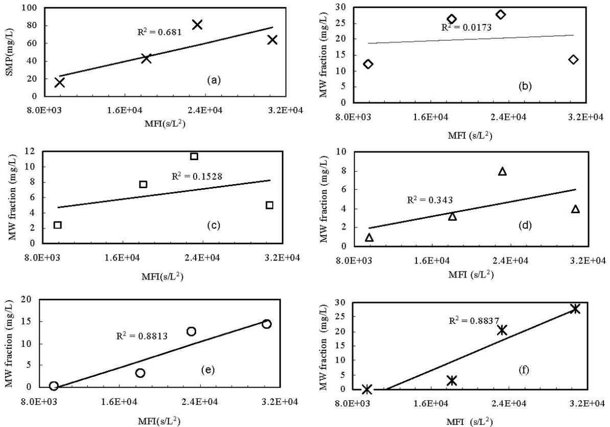
Fig. 6. Correlations between MFI and the concentrations of SMP or the concentrations of MW fraction: (a) SMP; (b) <1 kDa; (c) 1–3 kDa; (d) 3–10 kDa; (e) 10–100 kDa; (f) >100 kDa.
