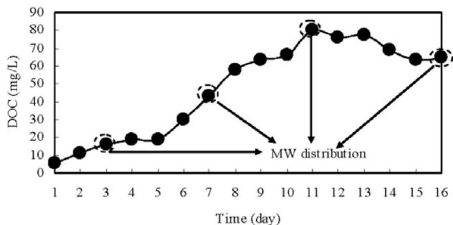
Fig. 2. Evolution of the SMP concentration against operation time (16 days).
