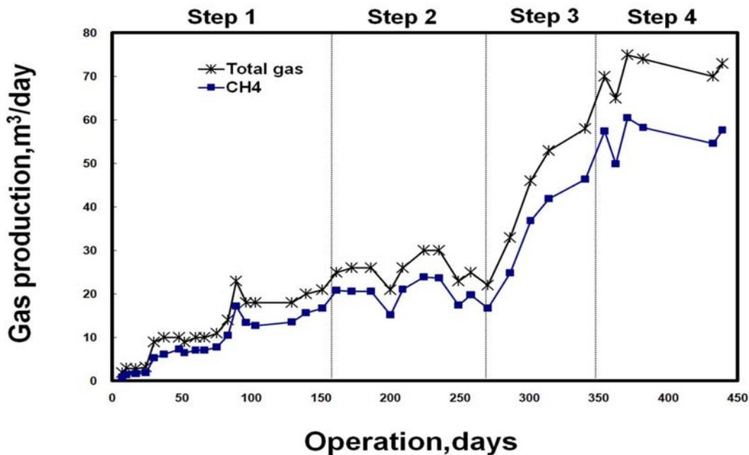
Fig. 7. Variation of biogas production in the UASB reactor.
