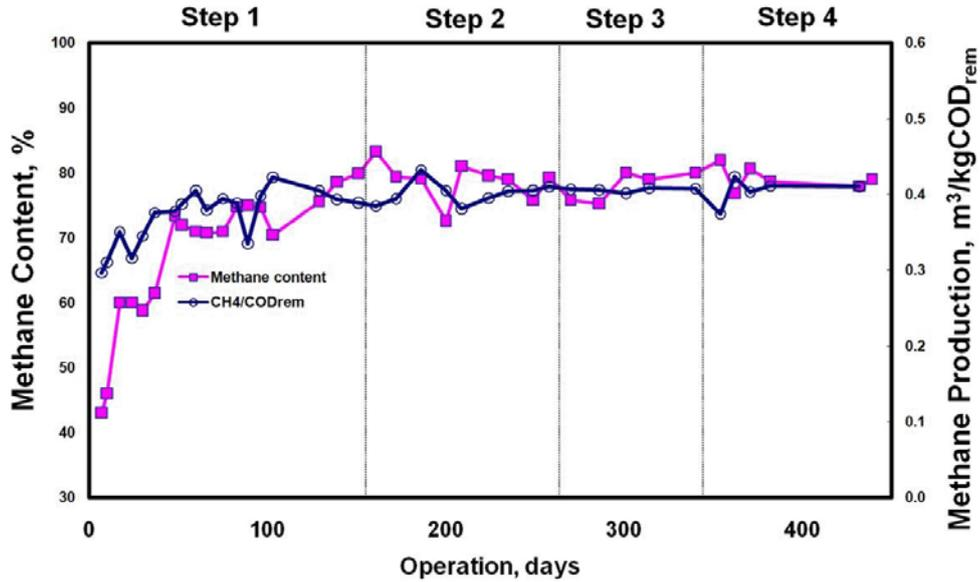
Fig. 8. Methane content and specific methane production rate.
