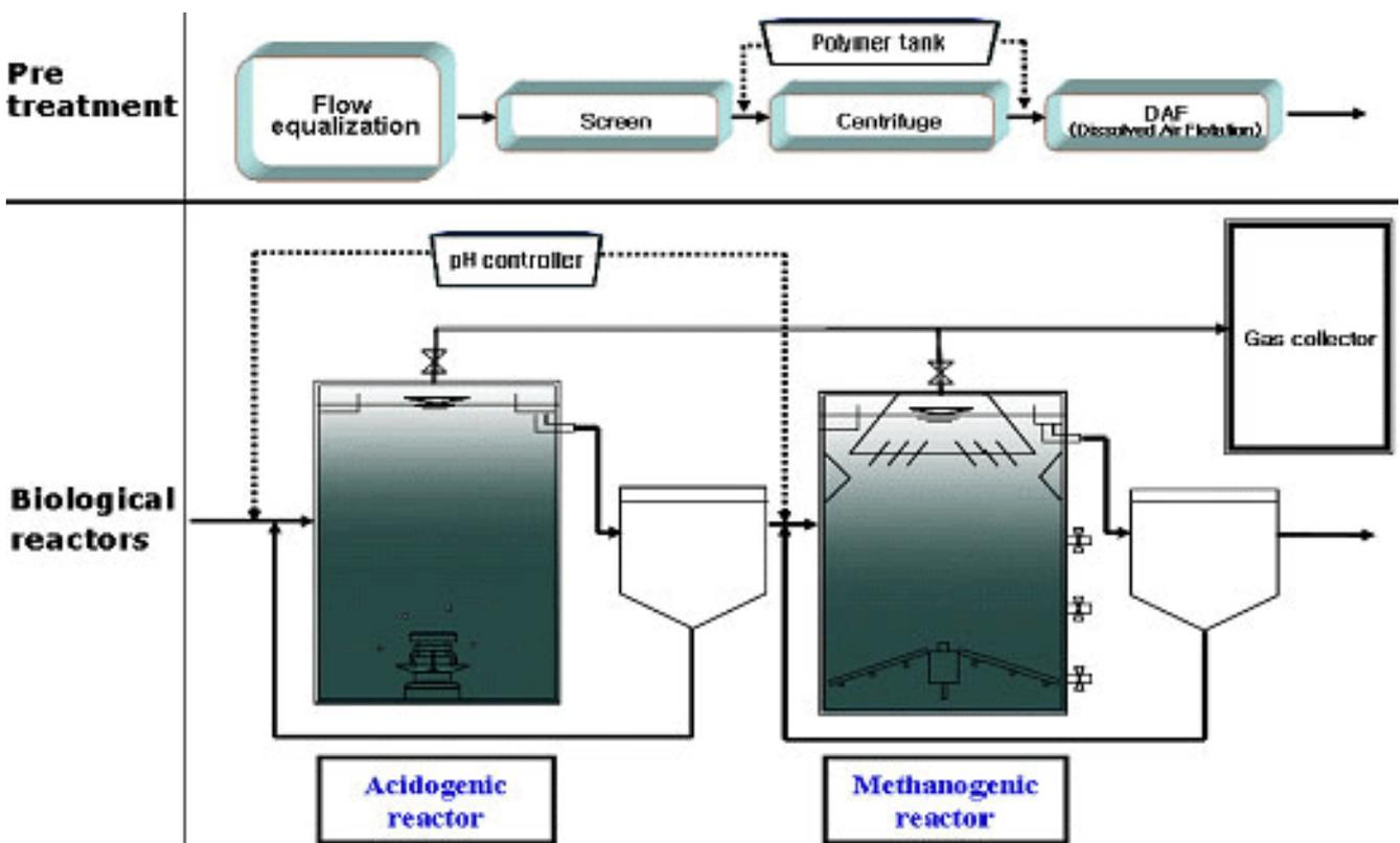
Fig. 1. Schematic diagram of two-phase anaerobic process.
