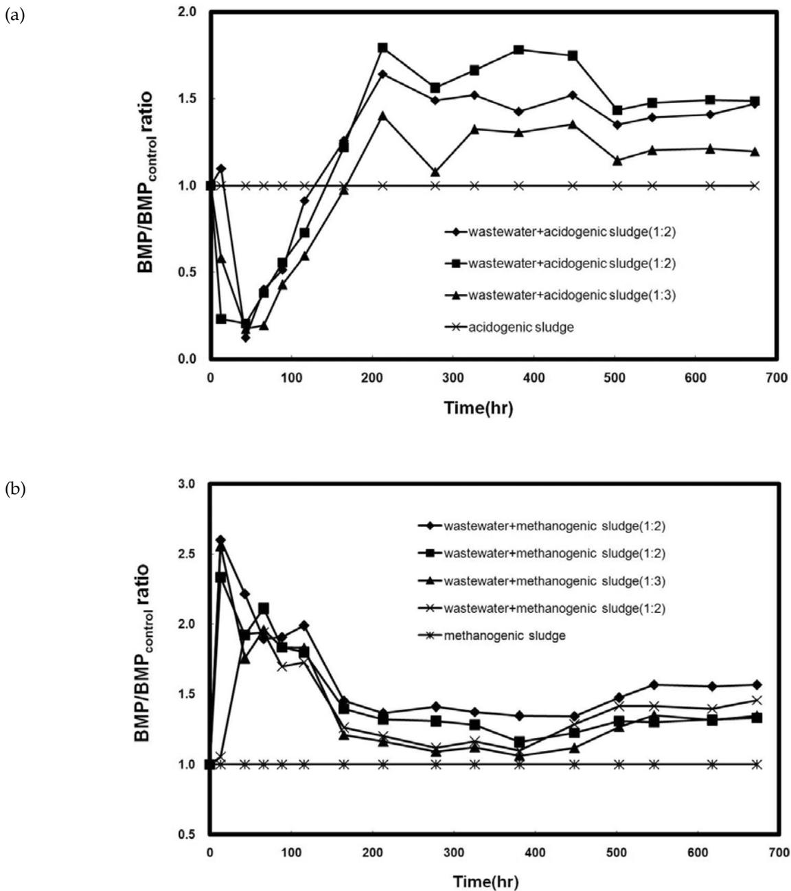
Fig. 2. (a) BMP/BMP<sub>control</sub> of acidogenic sludge. (b) BMP/BMP<sub>control</sub> of methanogenic sludge.
