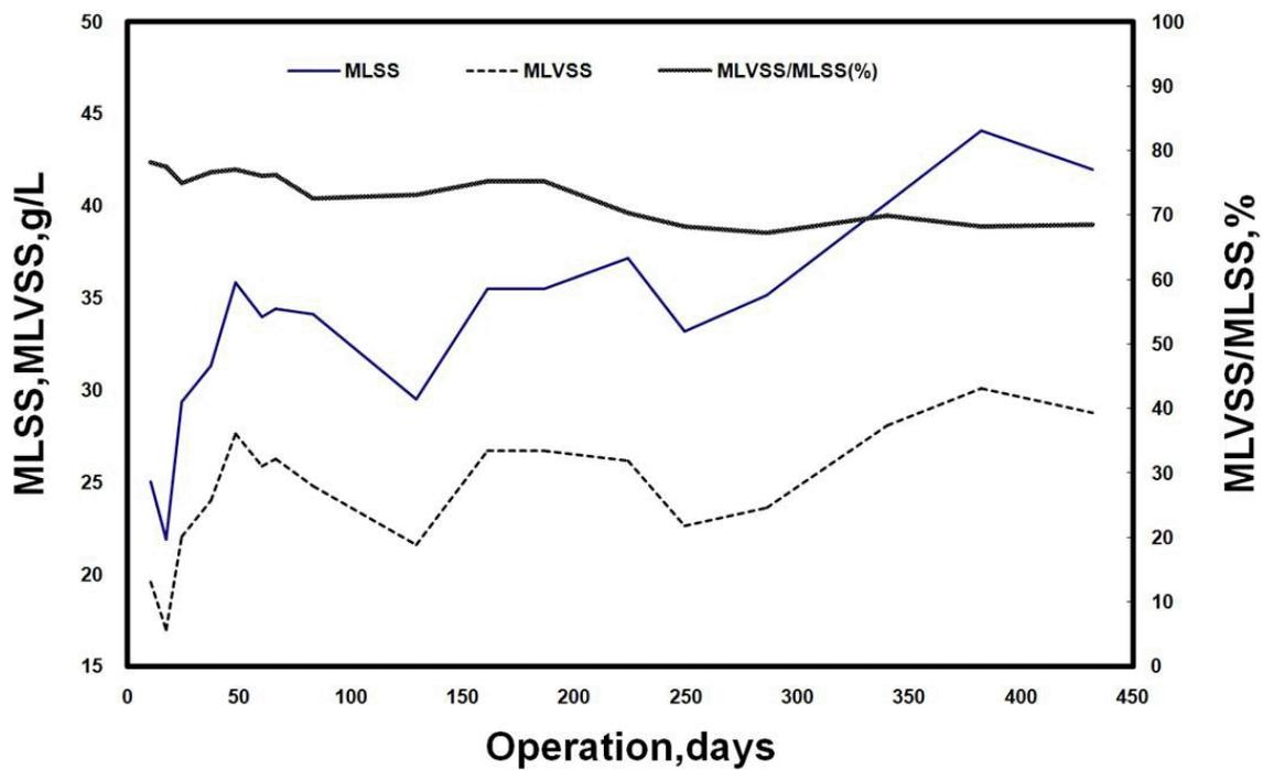
Fig. 10. Biomass concentration in the UASB reactor.
