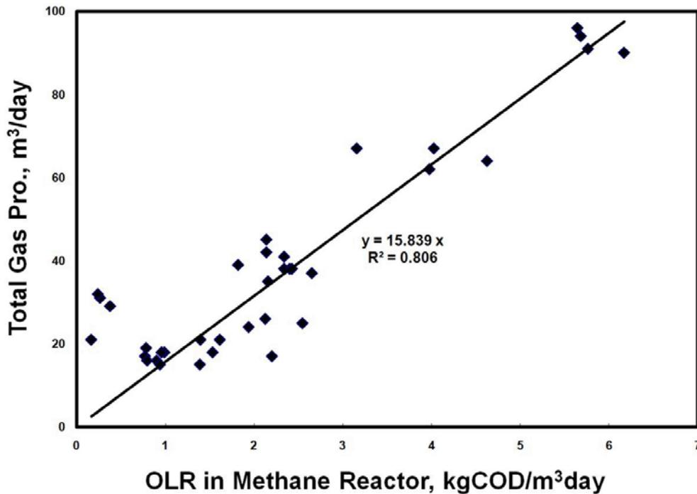
Fig. 9. Relationship between OLR and total gas production in UASB reactor.
