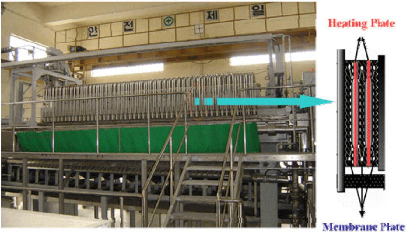
Fig. 2. Photograph of the full-scale thermal dehydrator.
