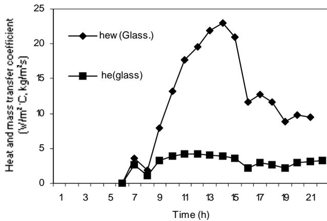
Fig. 5. Hourly variation of evaporative heat transfer coefficient and mass transfer coefficient for the glass cover.
