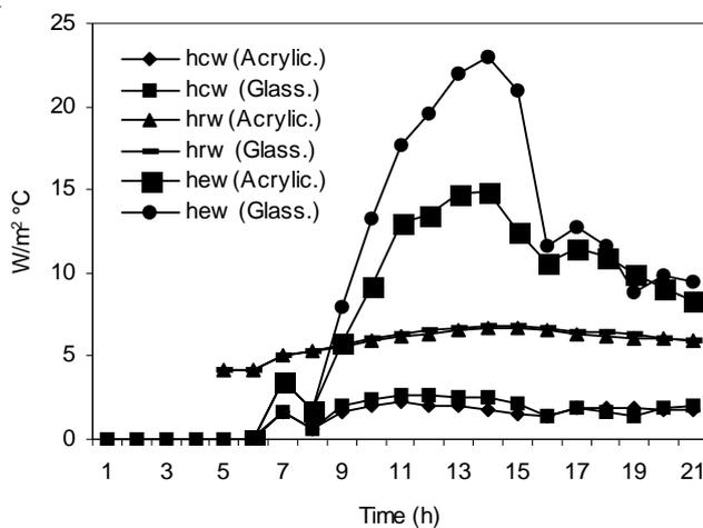
Fig. 7. Hourly variation of internal heat transfer coefficients.
