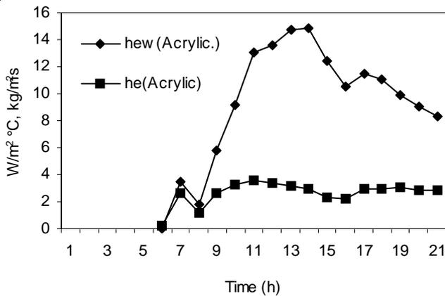
Fig. 6. Hourly variation of evaporative heat transfer coefficient and mass transfer coefficient for the acrylic cover.
