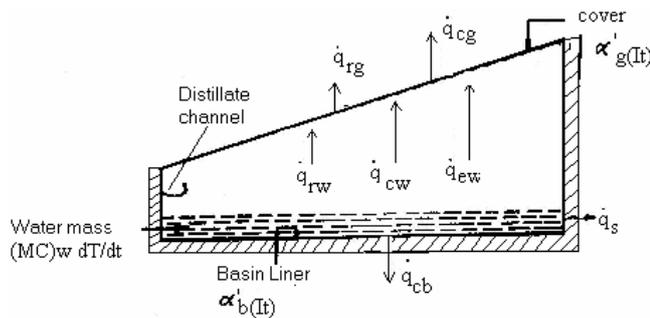
Fig. 1. Schematic diagram of heat transfer in a solar still.
